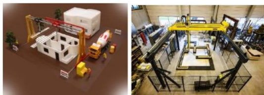
Fig. 5 Framed concrete 3D printers Source: https://www.tue.nl/en/university/departments/built-environment/research/research-programs/structural-design/research/research-areas/concrete-research-areas/3d-
