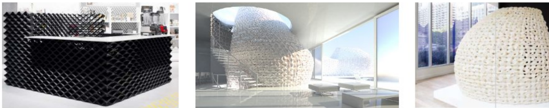
Fig. (1) Shows an interior space made of 3d printed mixture obtained by salt and glue constituting an efficient, translucent and inexpensive material https://www.archdaily.com/890494/interior-design-and-3d-
