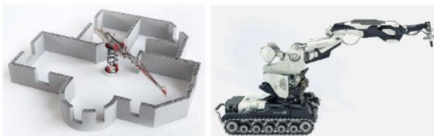
Fig. 6 Non-framed concrete 3D printers Source: https://3dprint.com/189228/cazza-3d-print-construction-robots/
