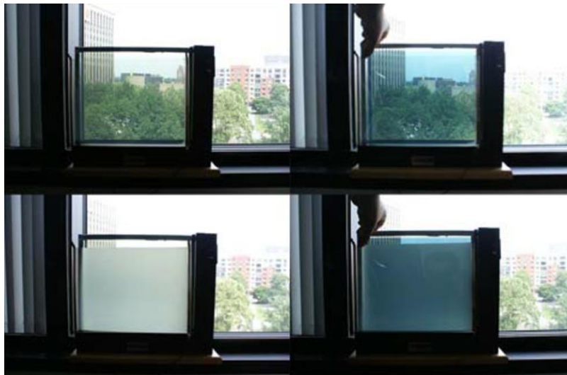
Figure 8. Demonstrates Glass Electrochromic Material (Telhan,2010)
