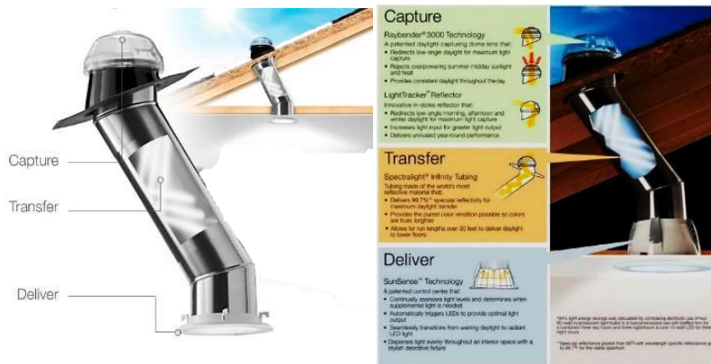
Figure 17 Components of natural tubular lighting units
