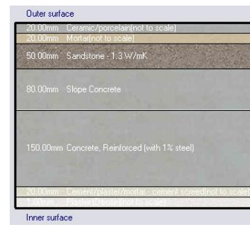
The base case materials of Roof
