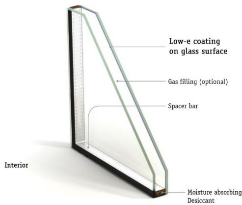
Figure 12: Layers of low-E glass • Reference:
