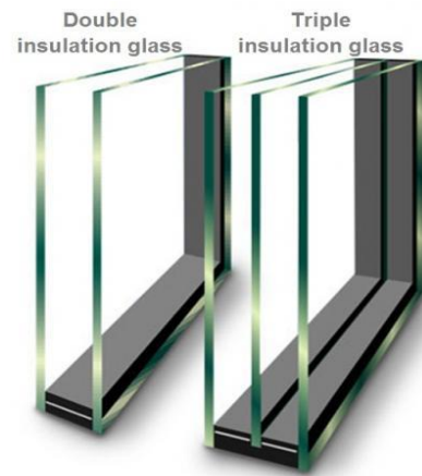
Figure 9: Double or triple insulation glass.
