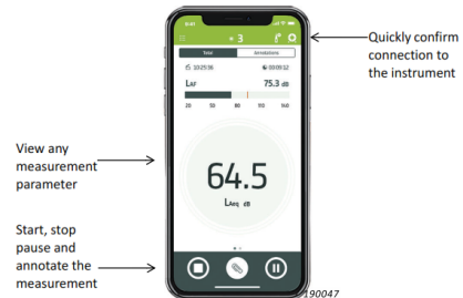
Fig. 3 Control, view and annotate measurements directly from your mobile phone
