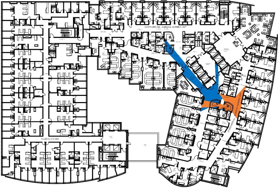
Figure 4- 81: H1-2D Isovist Analysis for Controllability (Nursing Unit 1) Source: By Researcher
