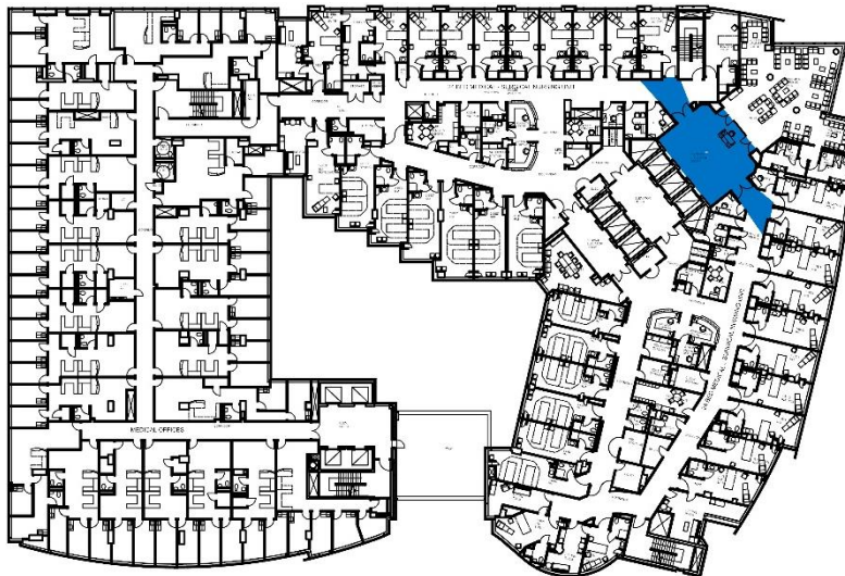
Figure 4- 77: H1-2D Isovist Analysis for Accessibility Source: By Researcher
