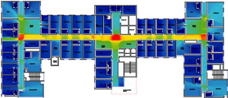
Figure 4- 74: H2 - Isovist field Analysis for Wayfinding Source: By Researcher
