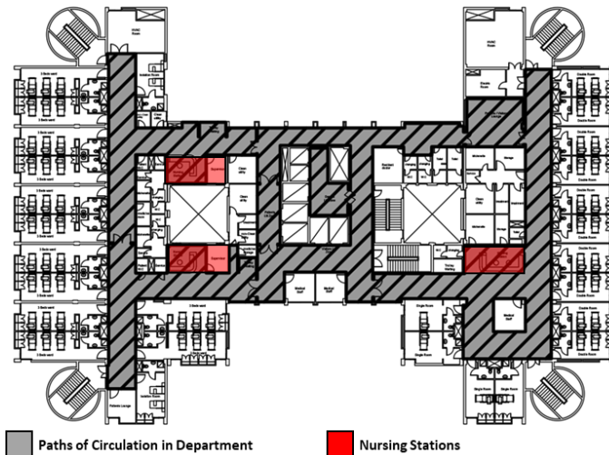
Figure 4- 3: El-Sheikh Zayed Al Nahyan Hospital - Inpatient Department Layout Configuration Source: By Researcher
