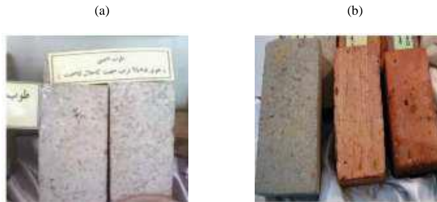
Figure (43): HBRC New Bricks (a) recycled clay brick (b) Cement dust brick
