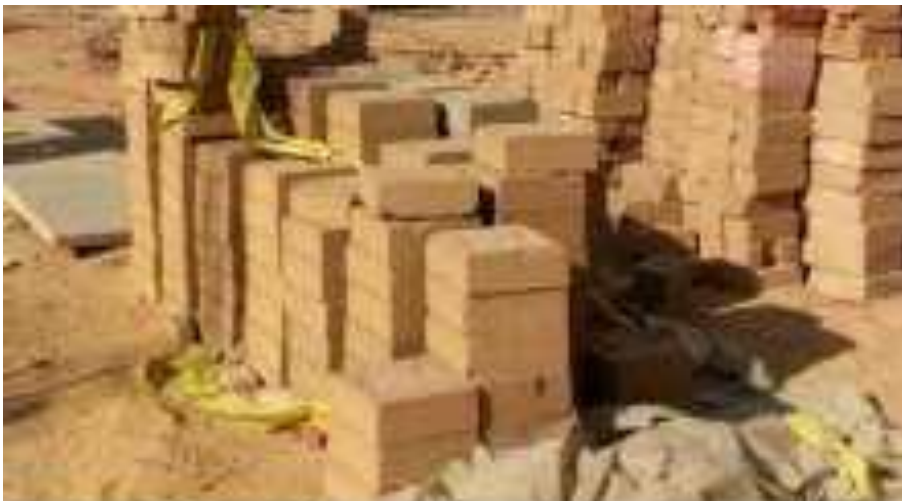
Figure (42): CEB Blocks are manufactured at the headquarters of the Housing and Building Research Center.
