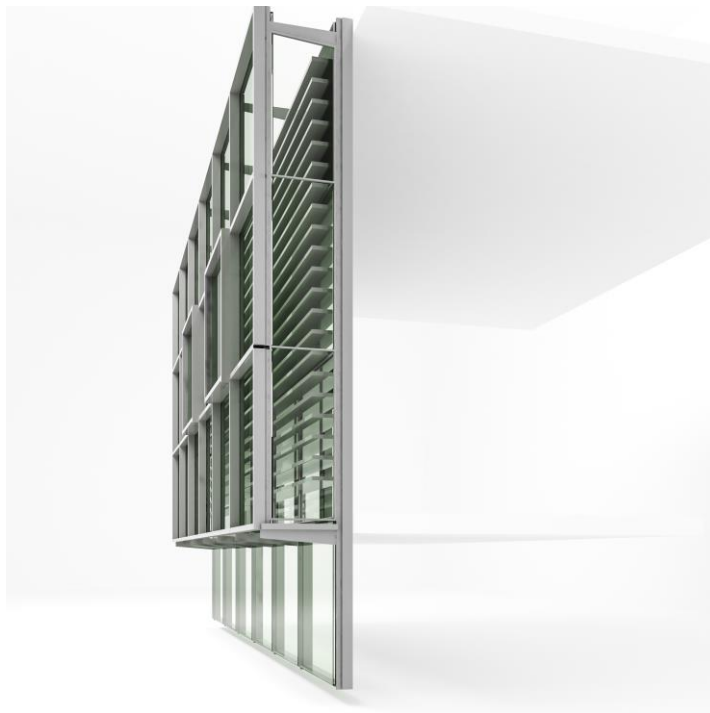
Figure 4-13- Model of Naturally Ventilated Wall with Shading Slats near Inner Skin
