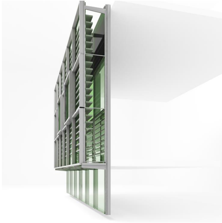
Figure 4-12- Model of Naturally Ventilated Wall with Shading Slats near Outer Skin
