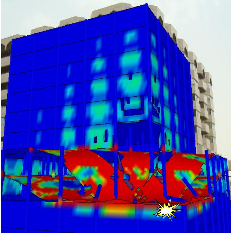
Fig. 10 Damages on the floor system of building for threat scenario – 1
