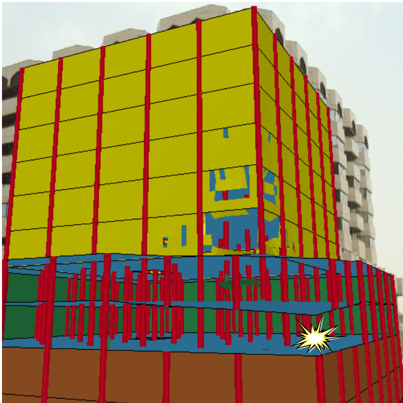
Fig. 7 Damage state of building at 2.80s for threat scenario – 1
