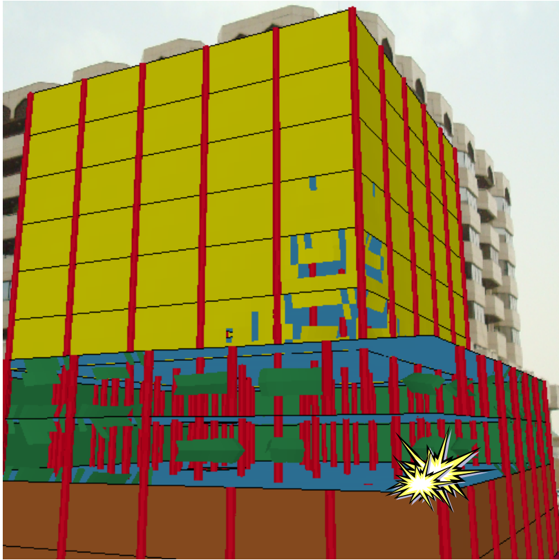
Fig. 6 Damage state of building at 2.55s for threat scenario – 1
