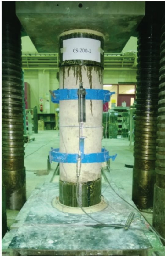
Figure 7. Instrumented column ready for testing.
