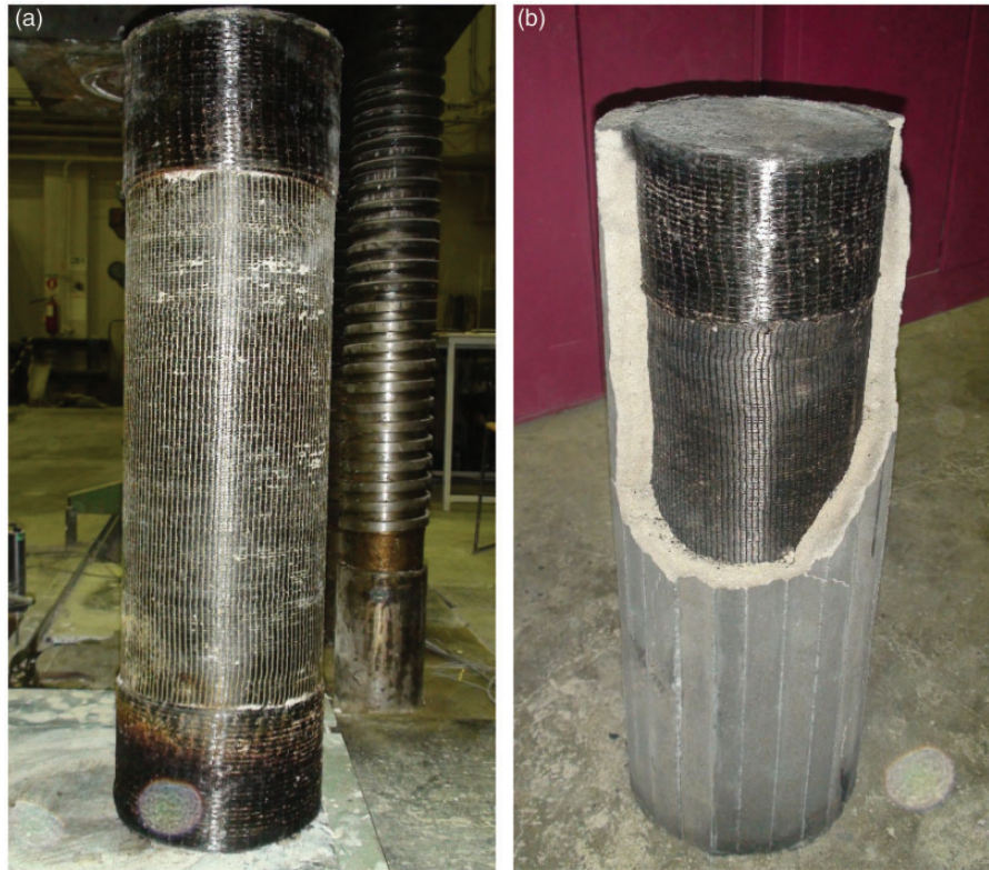
Figure 6. Insulated CFRP-strengthened columns after exposure for 3 h. (a) Insulated CFRP-wrapped column exposed to 500°C and (b) insulated CFRP-wrapped column exposed to 800°C.
