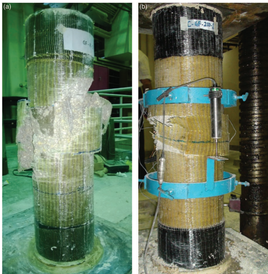
Figure 10. Typical failure modes for GFRP-strengthened specimens. (a) Room Temp. and (b) 200°C.
