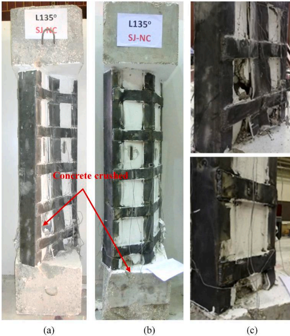
Fig. 13. Failure of specimen L135-SJ-NC: (a) Elevation view; (b) Rear view; (c) Close view.
