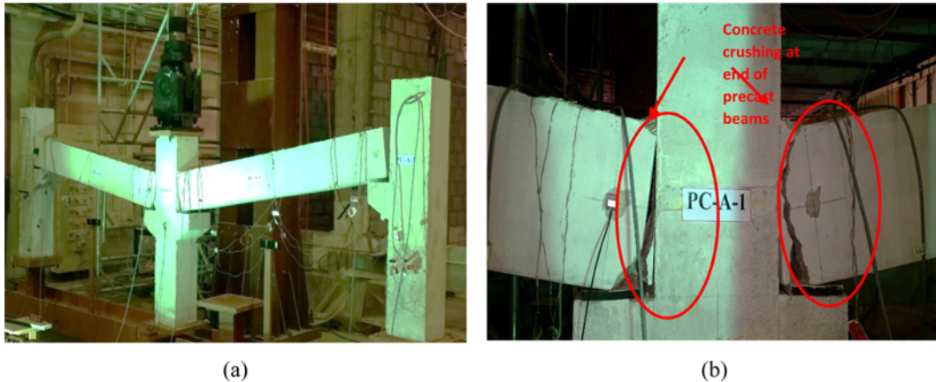
Fig. 10. Final Deformed Shape for PC-A Specimen at a Middle Column Displacement of 350 mm: (a) Final Deformed Shape, (b) Failure of Middle Joint
