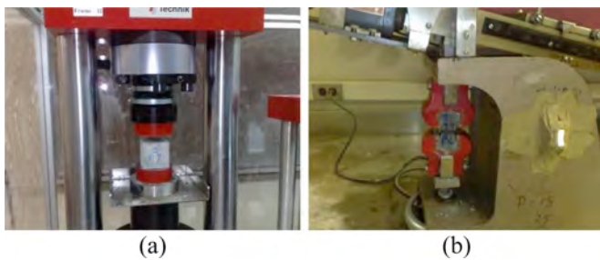
Fig. 7. Standard testing of mortar specimens [69]: (a) Cube specimens in compression; (b) Briquette specimens in tension.
