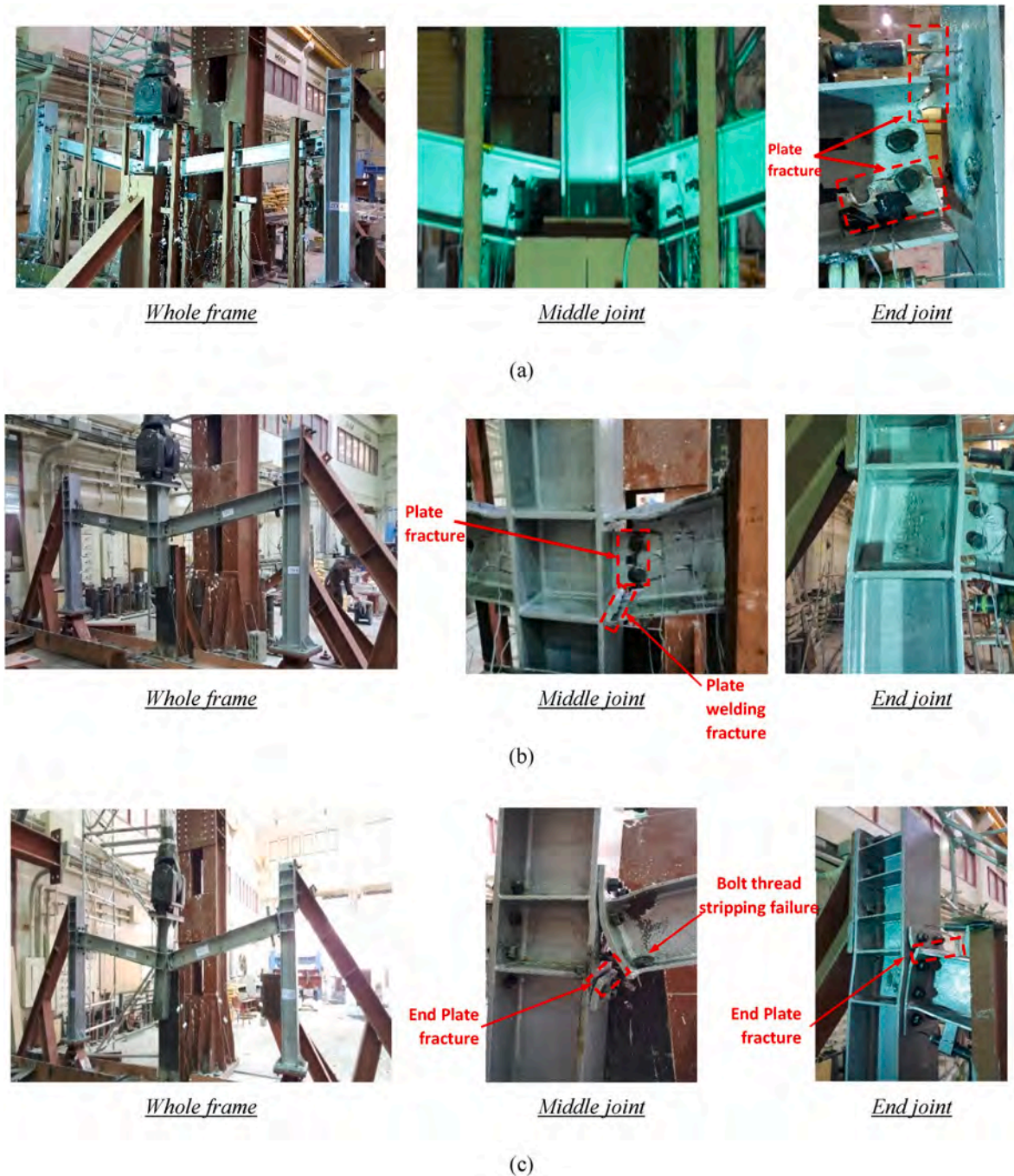
Fig. 4. Observed mode of failure for specimens tested in current study: (a) Specimen S-C; (b) Specimen WUF-FW; (c) Specimen 4 E-BUEEP-P.
