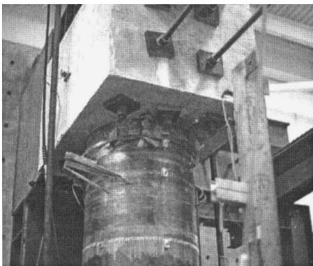
Fig. 7. Flexural failure of retrofitted circular Column CS-R4
