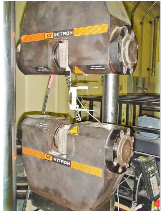
Fig. 4. Textile coupon under test (image by the authors)
