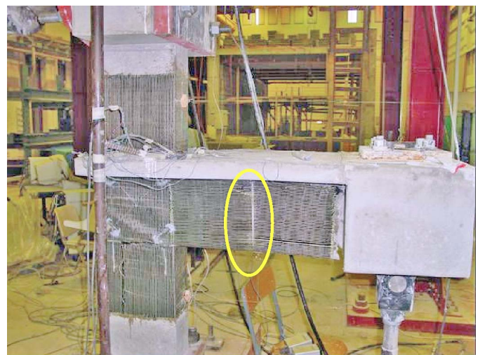
Fig. 19. Failure pattern of CFRP-strengthened specimen (image by the authors)
