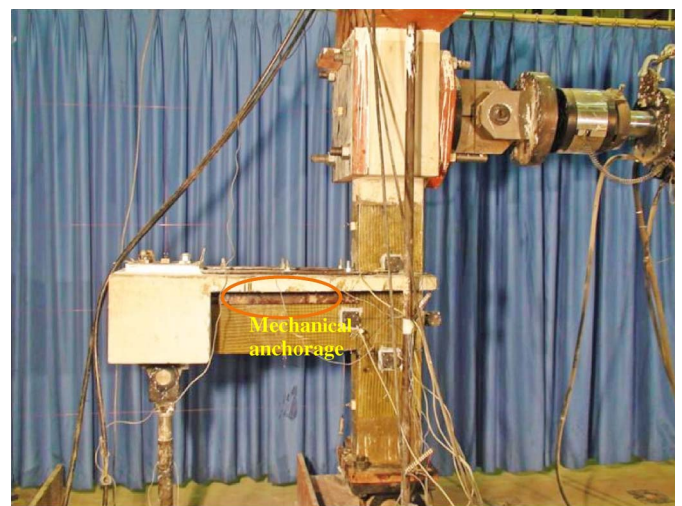
Fig. 8. Photo showing GFRP scheme applied to as-built exterior joint (image by the authors)
