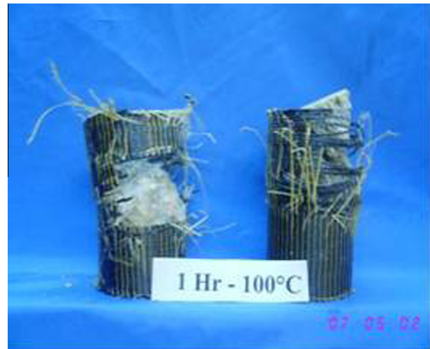
Fig. 8. Failure of the CFRP-confined specimens.
