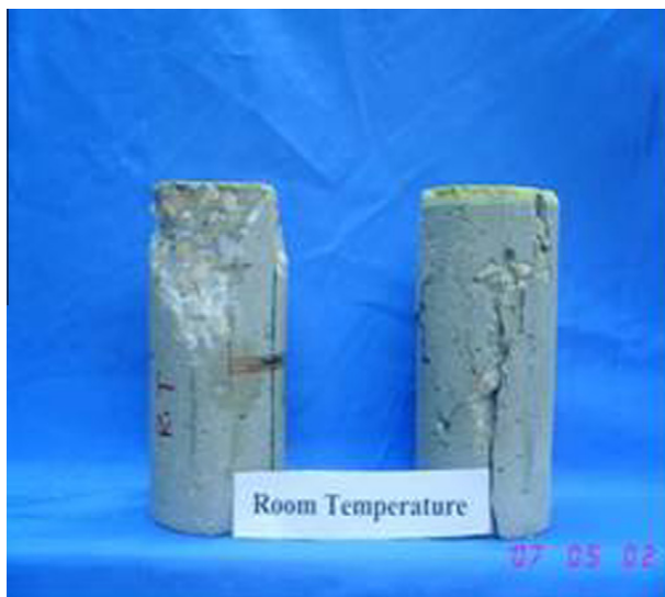
Fig. 4. Failure of the unconfined specimens.
