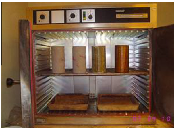
Fig. 1. Oven with concrete cylinders ready for heating.
