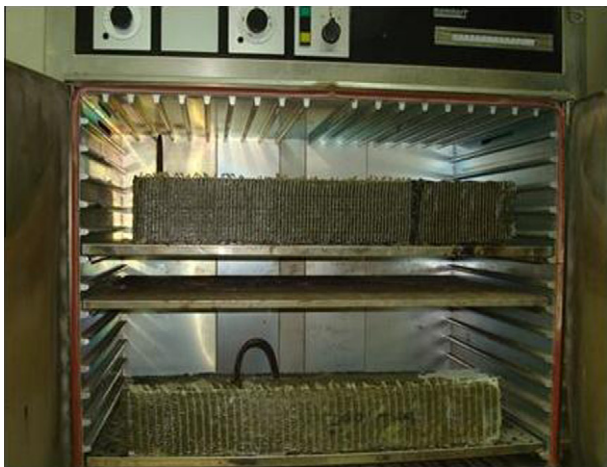
Fig. 19. Concrete prisms in the oven ready for heating.
