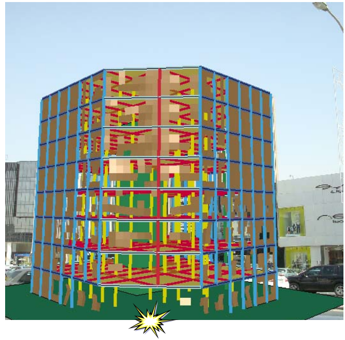
Fig. 8 Damage state of building at 3.1s
