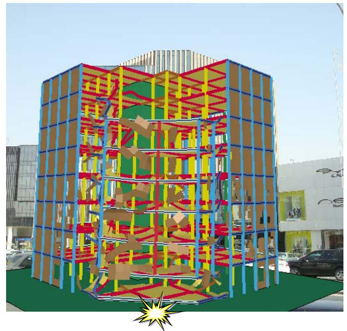
Fig. 9 Partial collapse of the building at 6s
