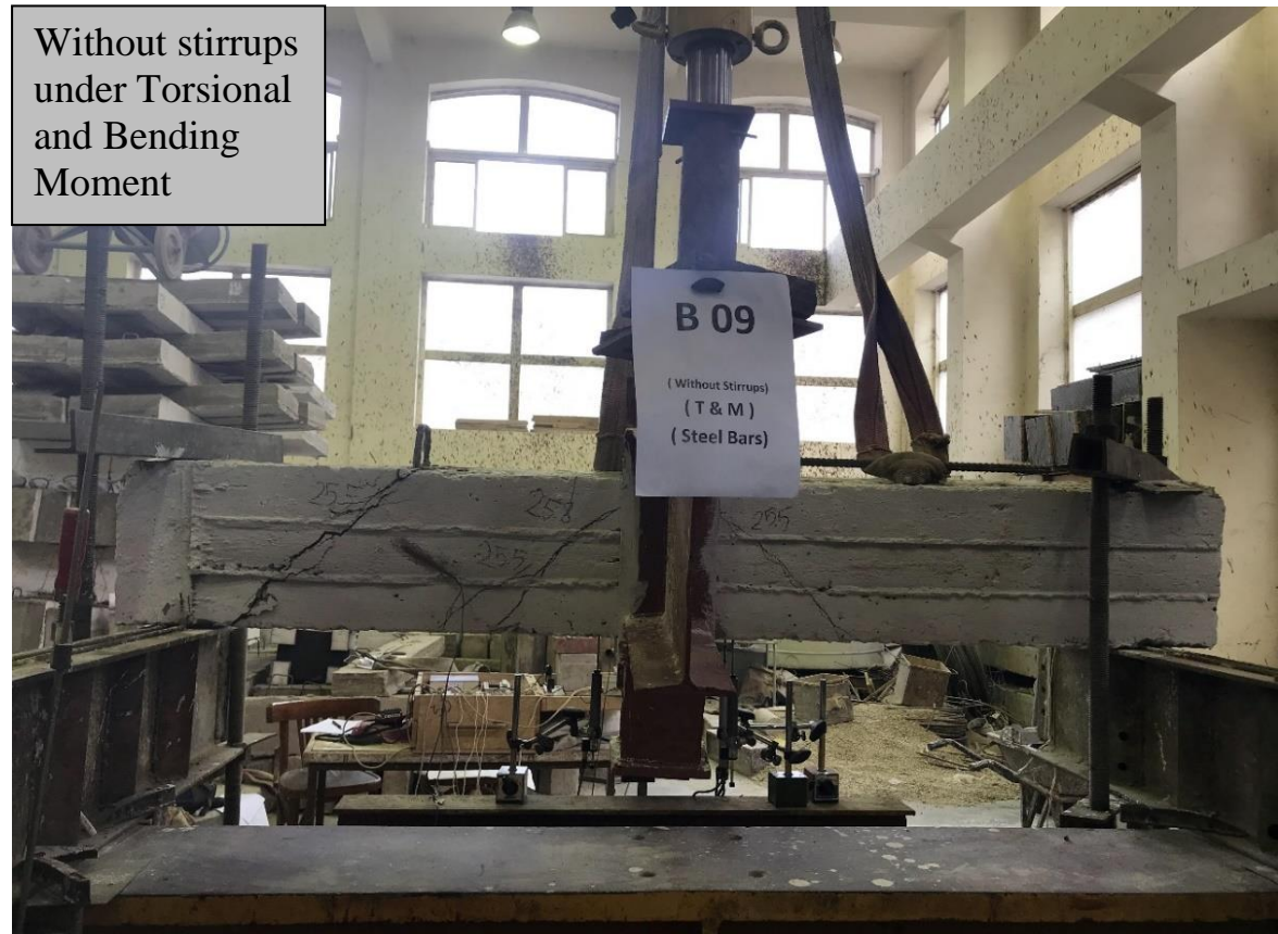
Figure (5-30) Cracks Pattern for Specimens B8 and B9.
