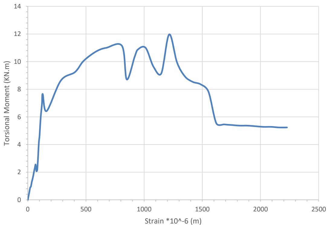
Figure (4- 76): Torsional Moment-Strain Curve for the Concrete at Quarter of Span Zone for Specimen B9.
