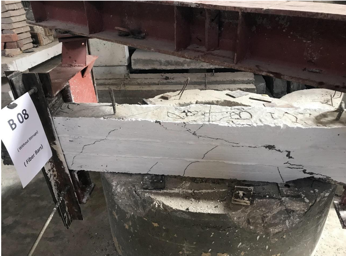
Figure (4-64-b): Cracks Pattern for the Second Side of Specimen B8.
