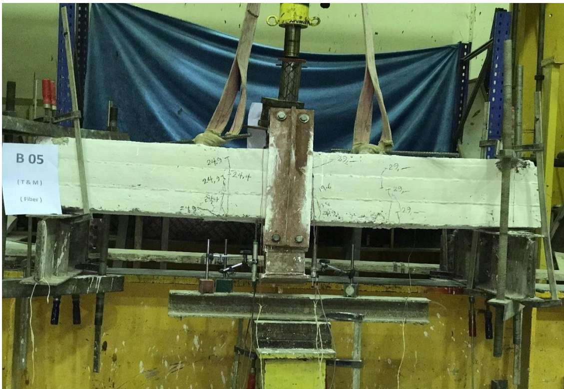
Figure (4-38-b): Cracks Pattern for the second side of Specimen B5.
