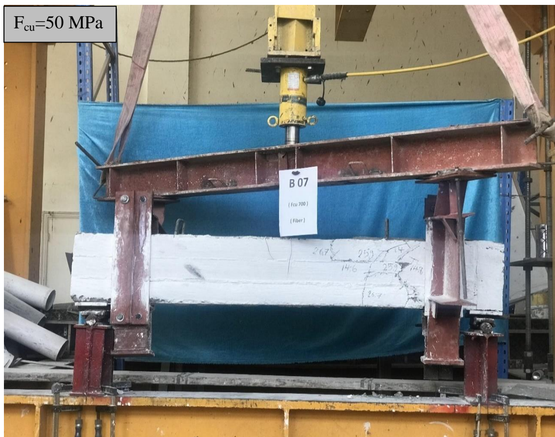
Figure (5-25): Cracks Pattern for Specimens B2 and B7.
