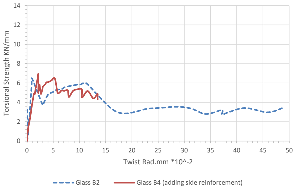
Figure (5-15): Twist-Torsional Moment Curve for B2 and B4.
