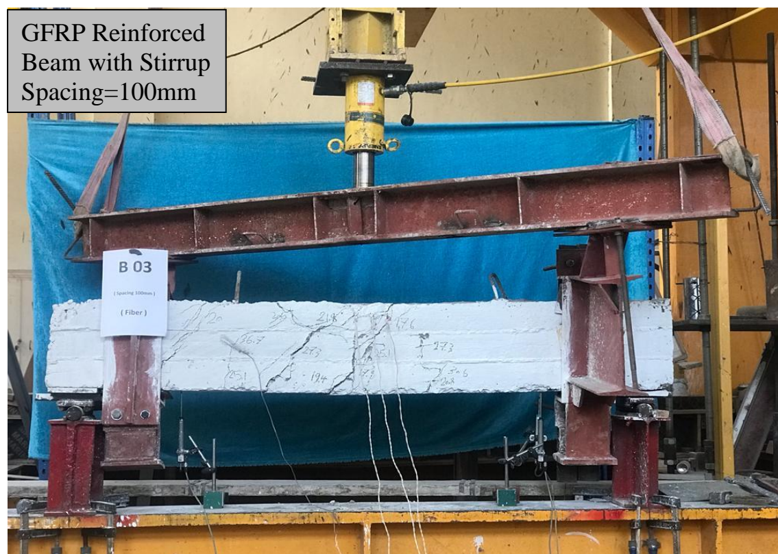
Figure (5-9): Cracks Pattern for Specimens B2 and B3.
