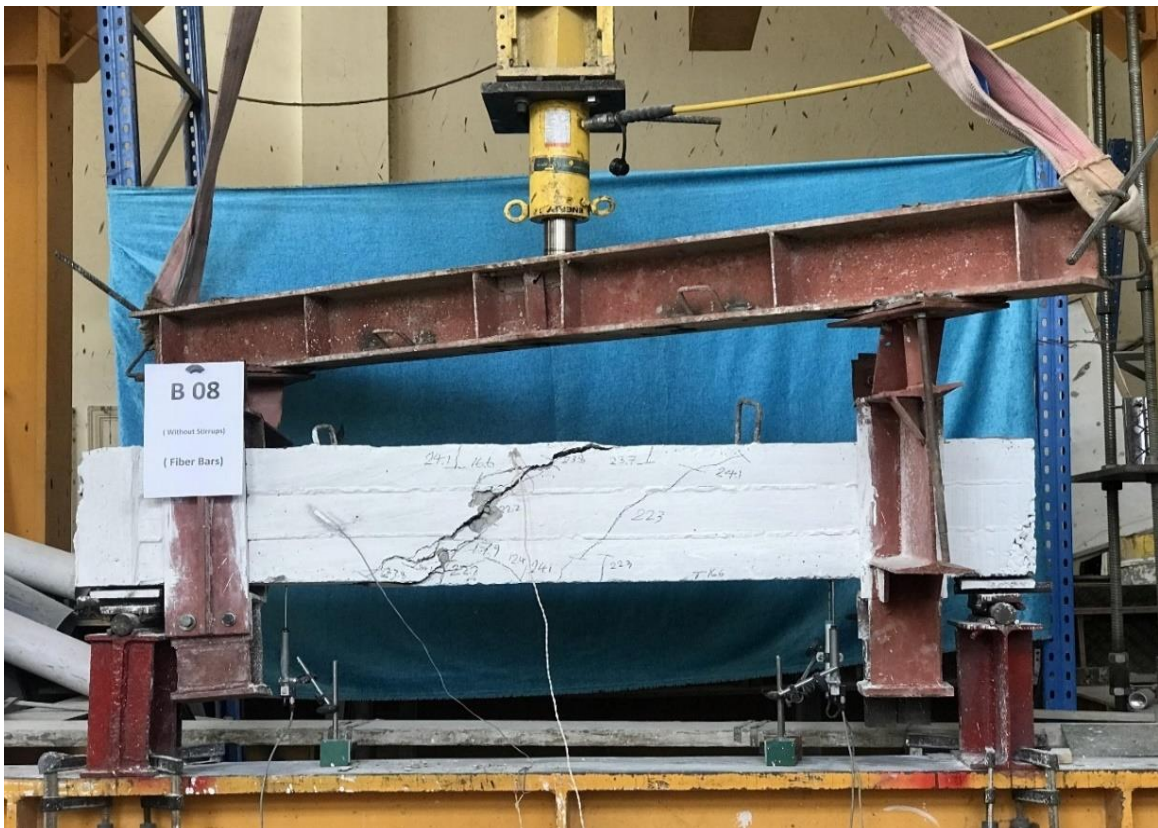
Figure (4-64-a): Cracks Pattern for the First Side of Specimen B8.
