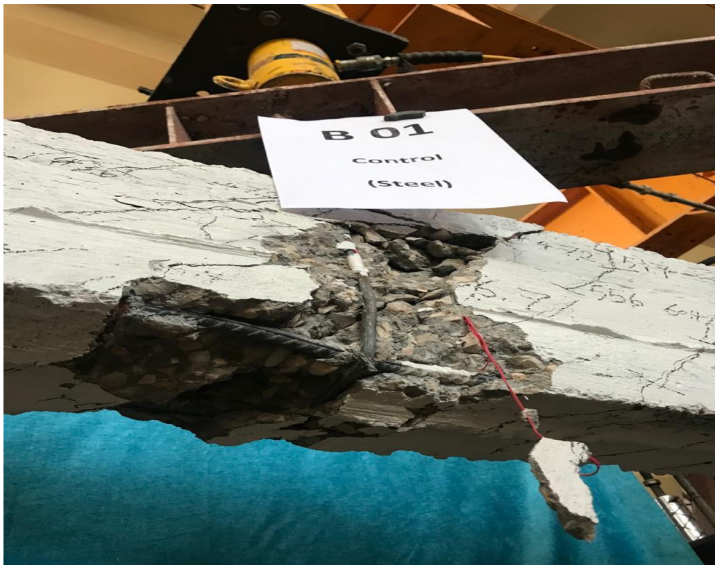
Figure (4-1): Cracks Pattern for Specimen B1.
