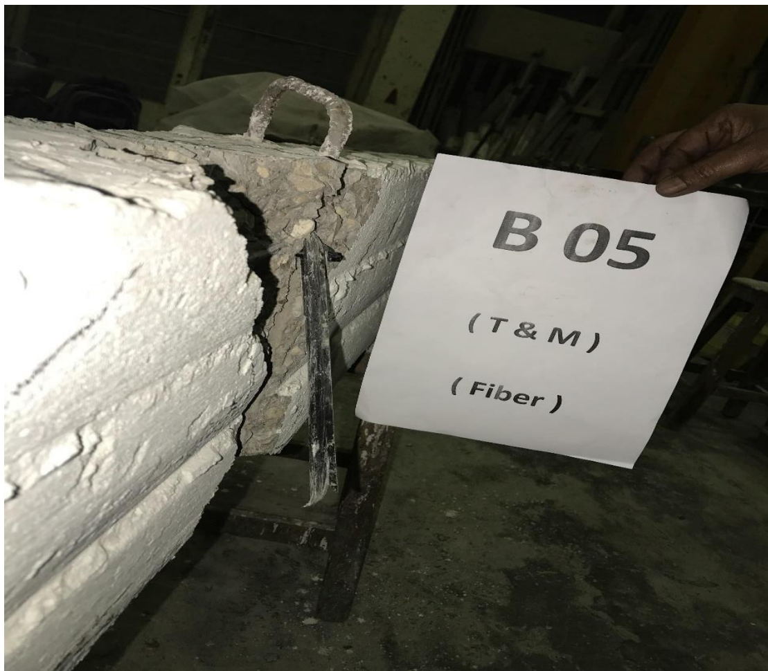
Figure (4-38-d) Rupture of Stirrup of Specimen B5.
