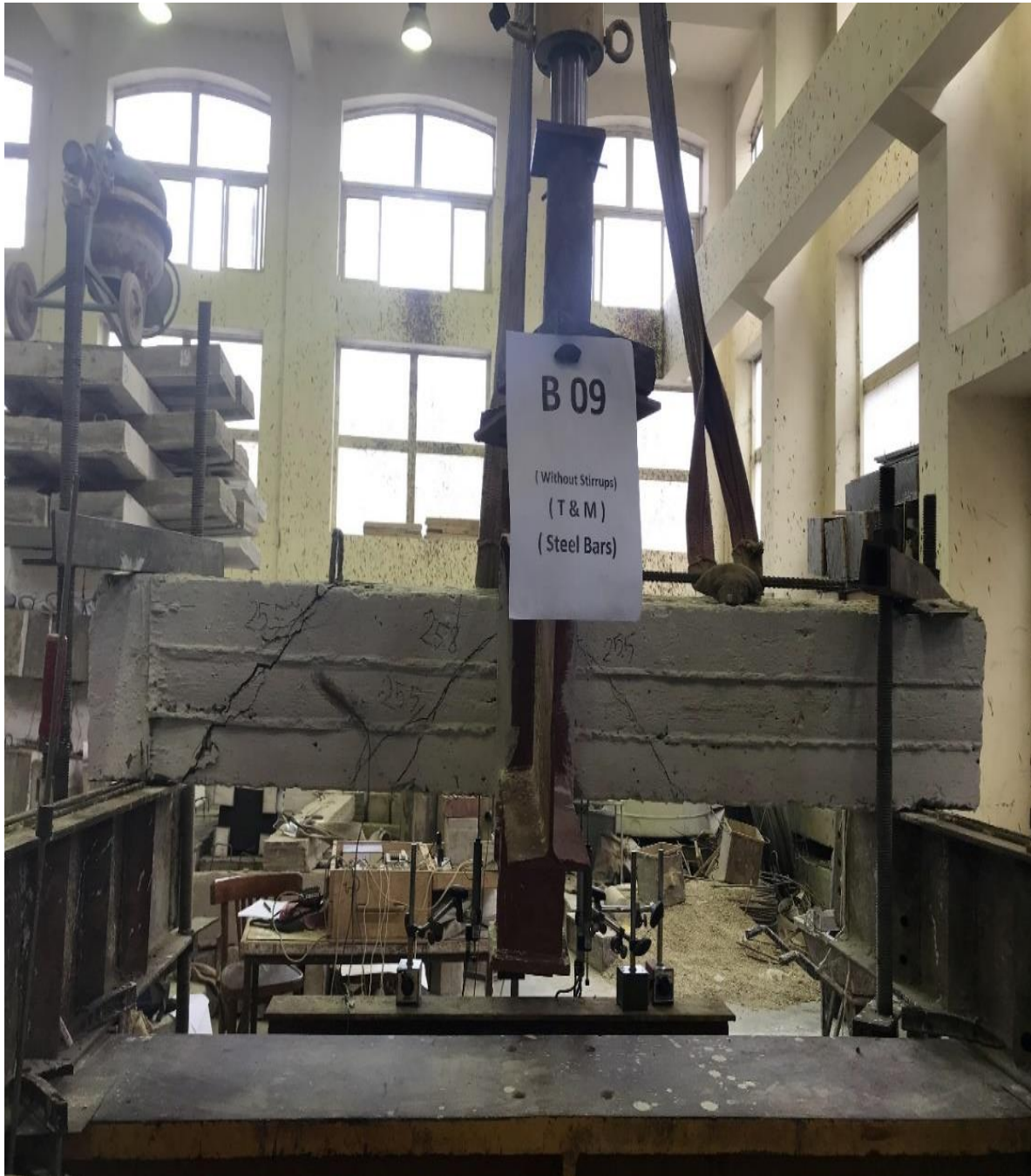
Figure (4-71-a): Cracks Pattern for Specimen B9.
