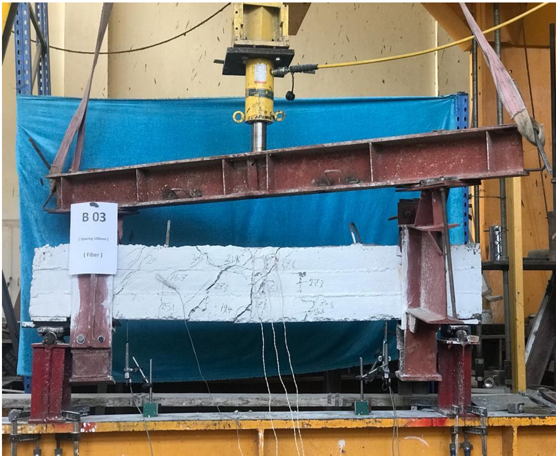
Figure (4-22-a): Cracks Pattern for Specimen B3.
