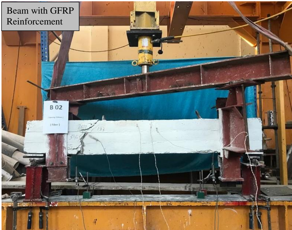
Figure (5-1): Cracks Pattern for Specimens B1 and B2.
