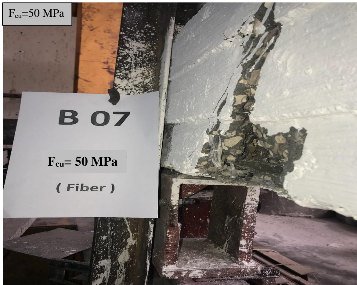
Figure (5-26-b) Rupture in Stirrups for Specimen B7.
