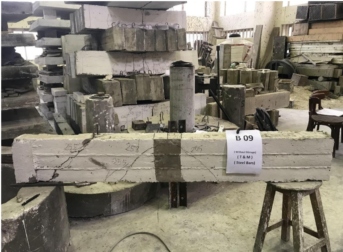
Figure (4-71-b): Cracks Pattern for Specimen B9.
