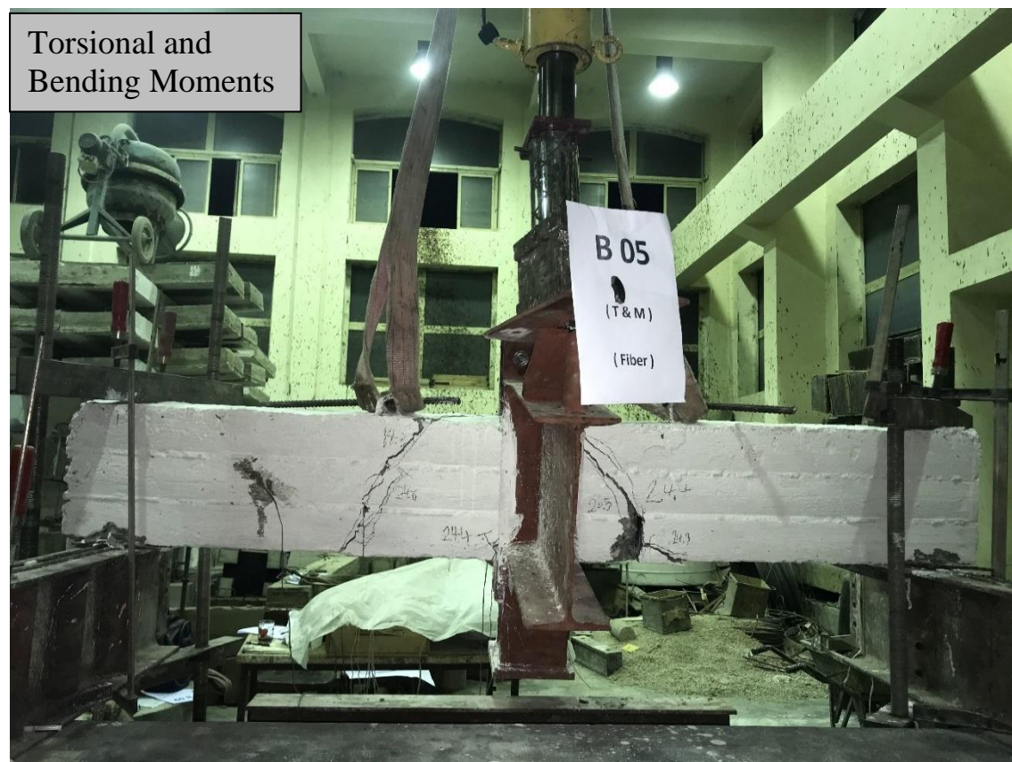
Figure (5-17): Cracks Pattern for Specimens B2 and B5
