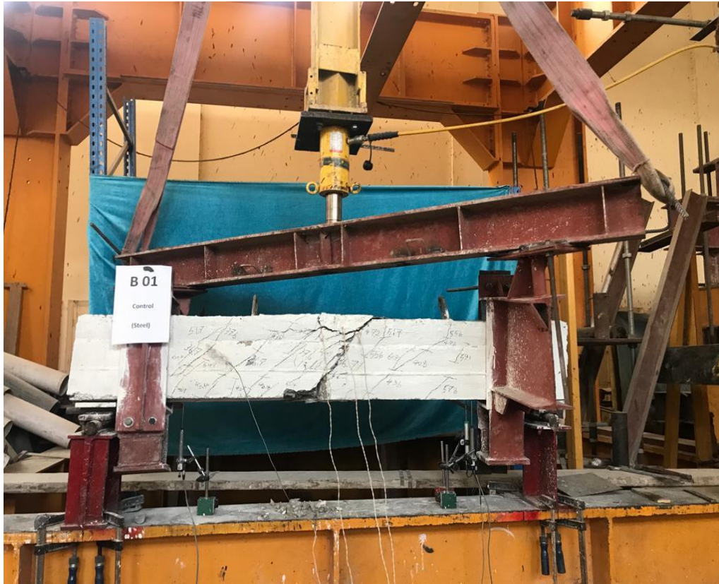
Figure (4-1): Cracks Pattern for Specimen B1.
