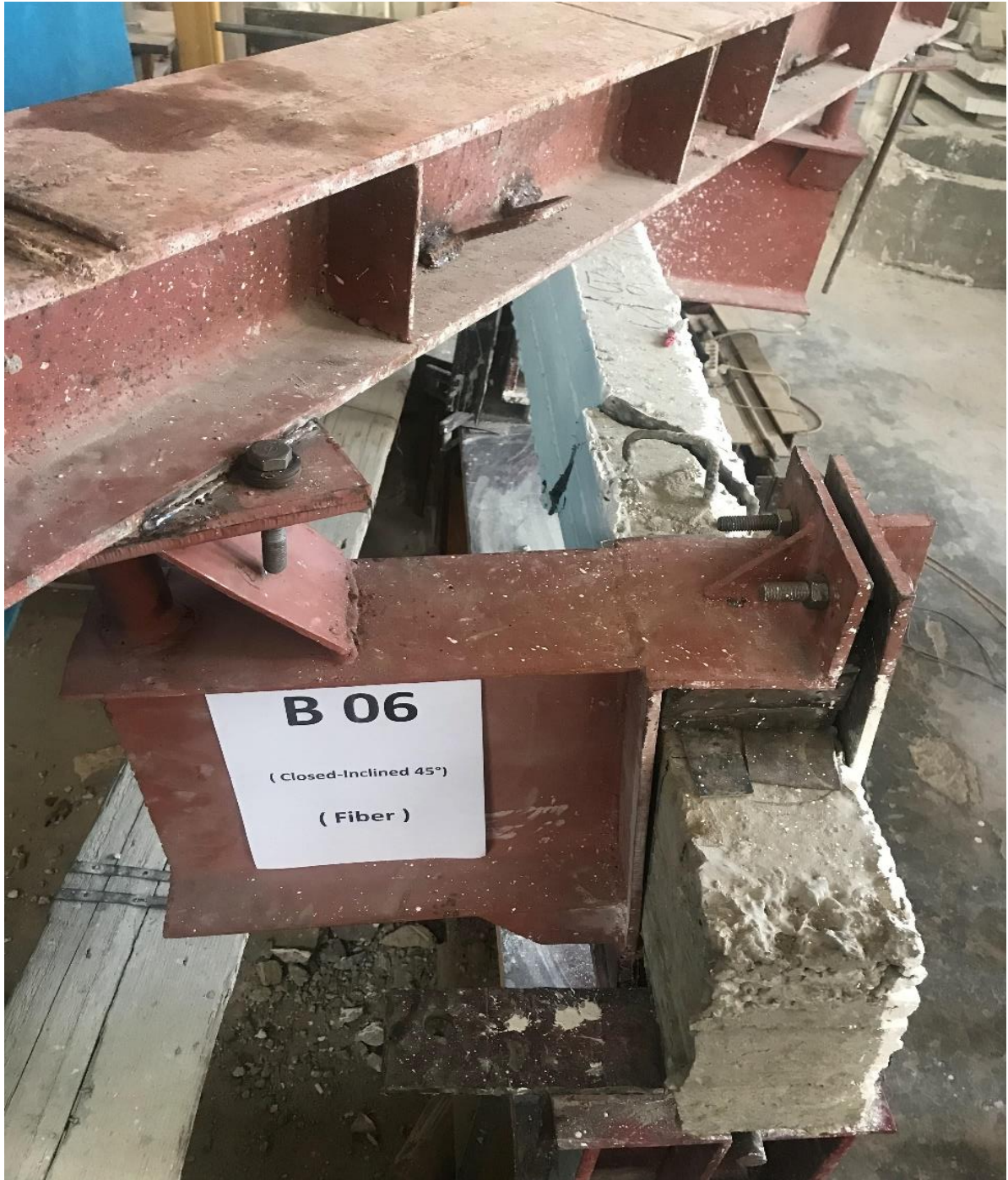
Figure (5-45-b): Cracks Pattern for the Top Side of Specimen B6.
