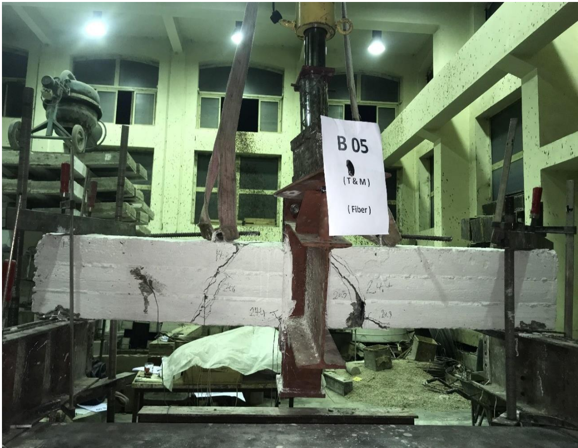
Figure (4-38-a): Cracks Pattern for the First Side of Specimen B5.
