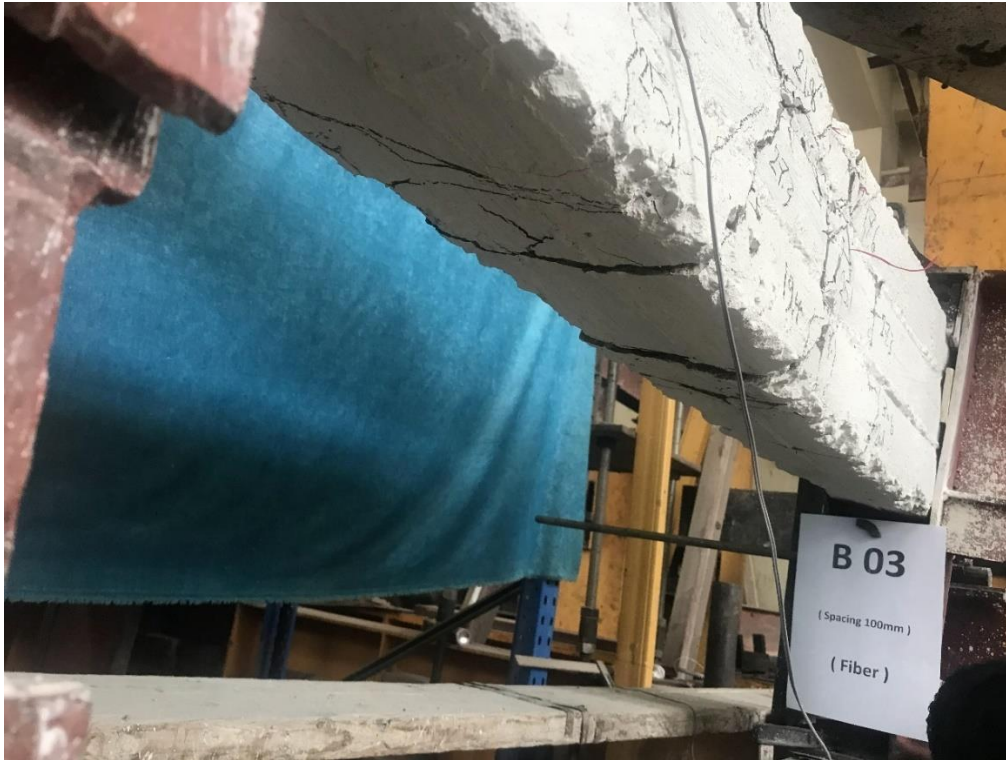
Figure (4-22-b): Cracks Pattern of Bottom Side for Specimen B3.
