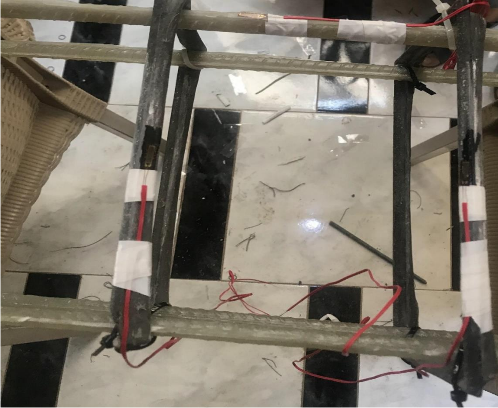
Figure (3-16): Reinforcement Electrical Resistance Strain
