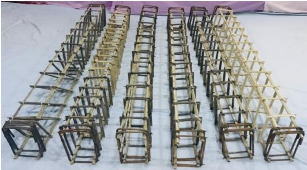
Figure (3-8): GFRP Reinforcement Details of Beams.
