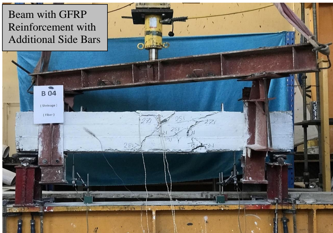
Figure (5-13): Cracks Pattern for Specimens B2 and B4.
