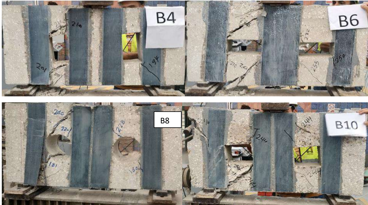
Figure (5-4): Crack patterns for beams strengthened with vertical BFRP strips.
