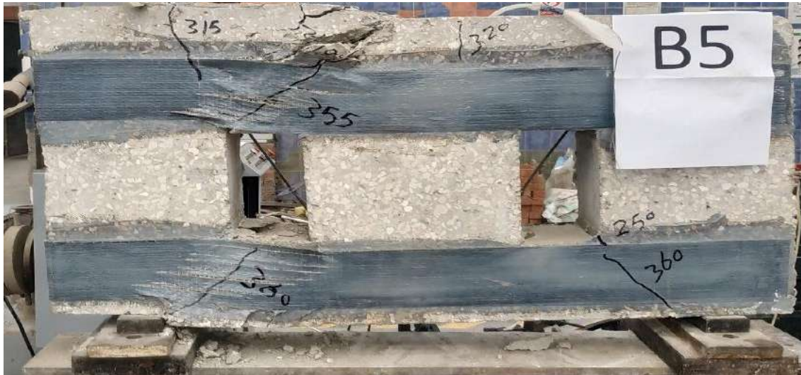
Figure (4-5): Crack pattern of (B5) at failure
