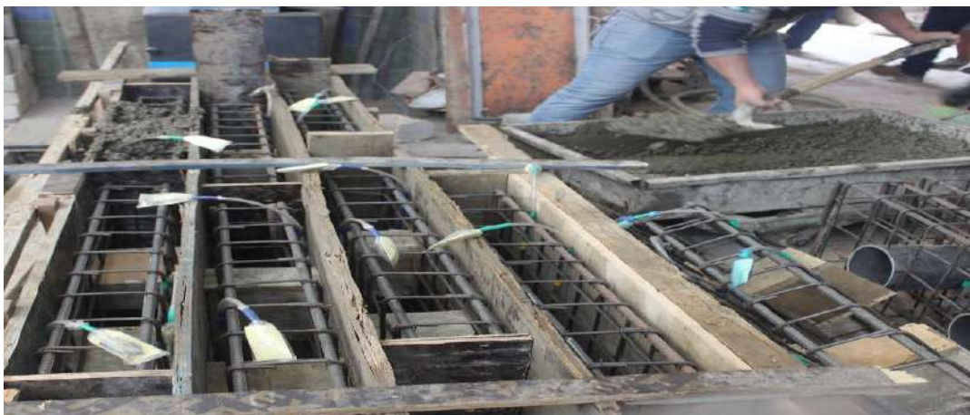
Figure (3-16): Casting of specimens
