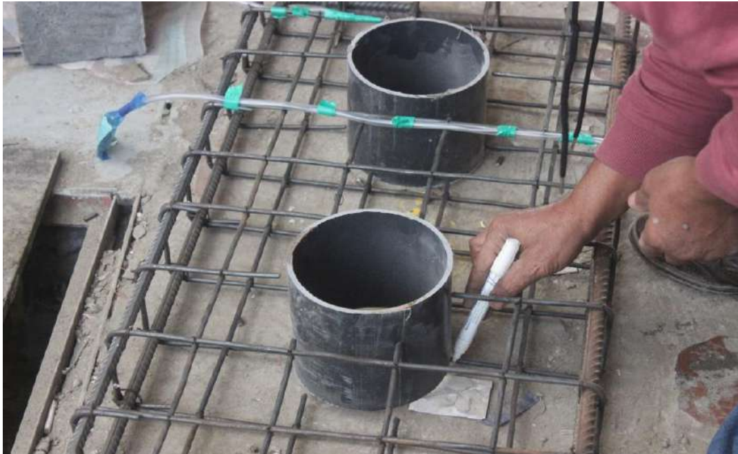
Figure (3-12): Preparing of the specimens for casting.
