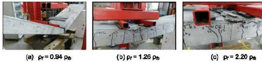
Figure (2-16): Flexure specimens at the conclusion of the test, High, C. et al. , [33]
