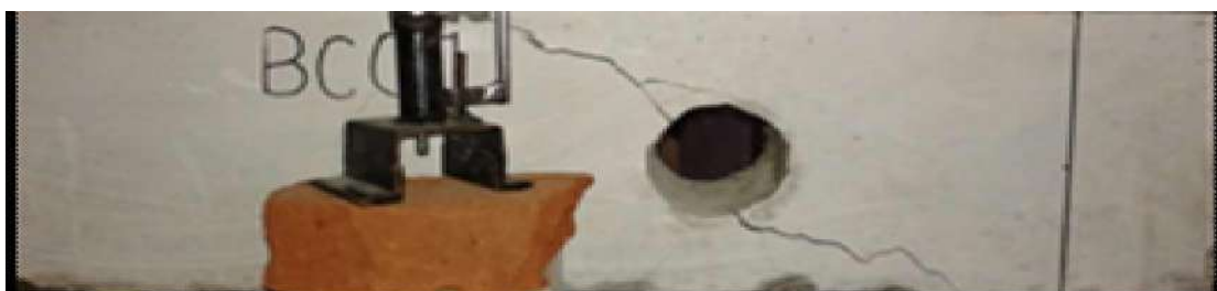
Figure (2-21): Unstrengthen beam with one circular opening. [38]
