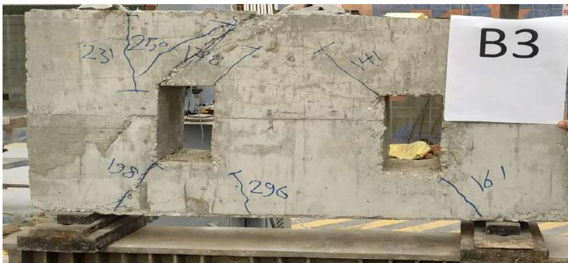
Figure (4-3): Crack pattern beam at failure (B3)
