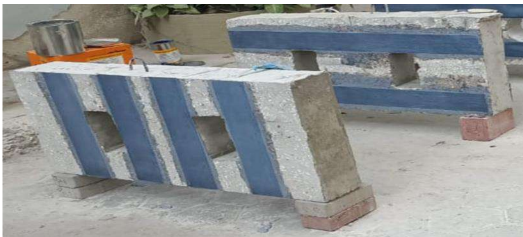
Figure (3-26): The final strengthened deep beams.
