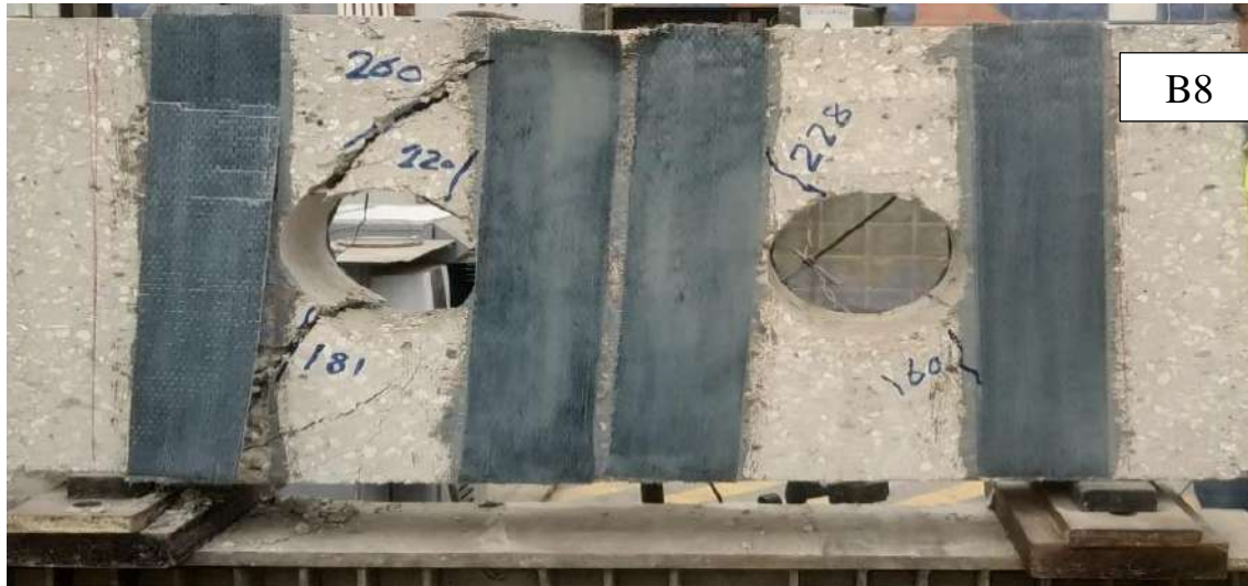
Figure (4-8): Crack pattern of beam B8 at failure
