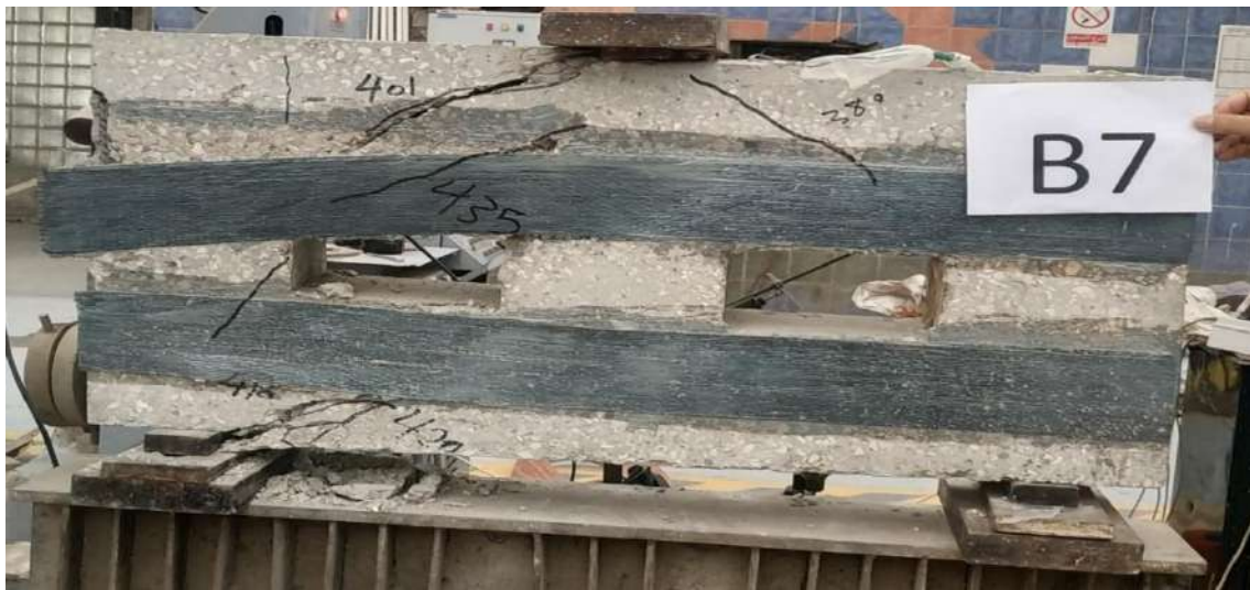
Figure (4-7): Crack pattern of beam B7 at failure
