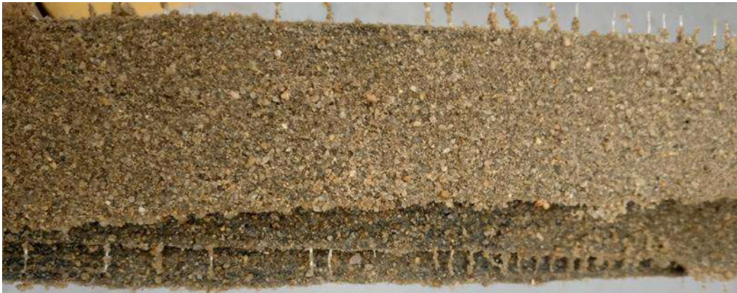
Figure (3-9): The specimen of basalt fiber roughed with sand
