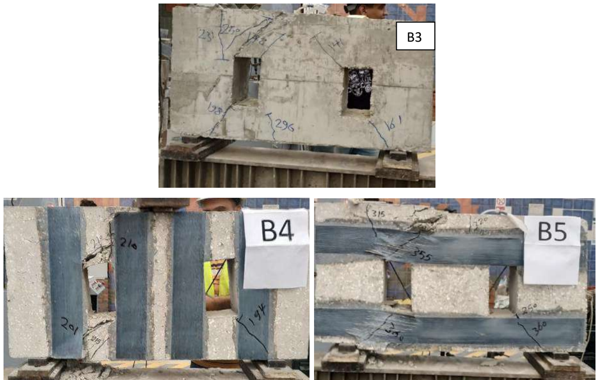
Figure (5-2): Crack pattern of deep beams with vertical rectangle openings
