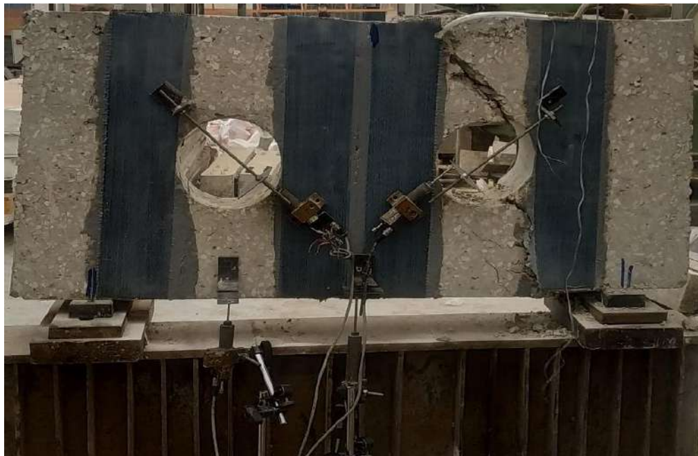
Figure (3-28): The location of deflection measurements.
