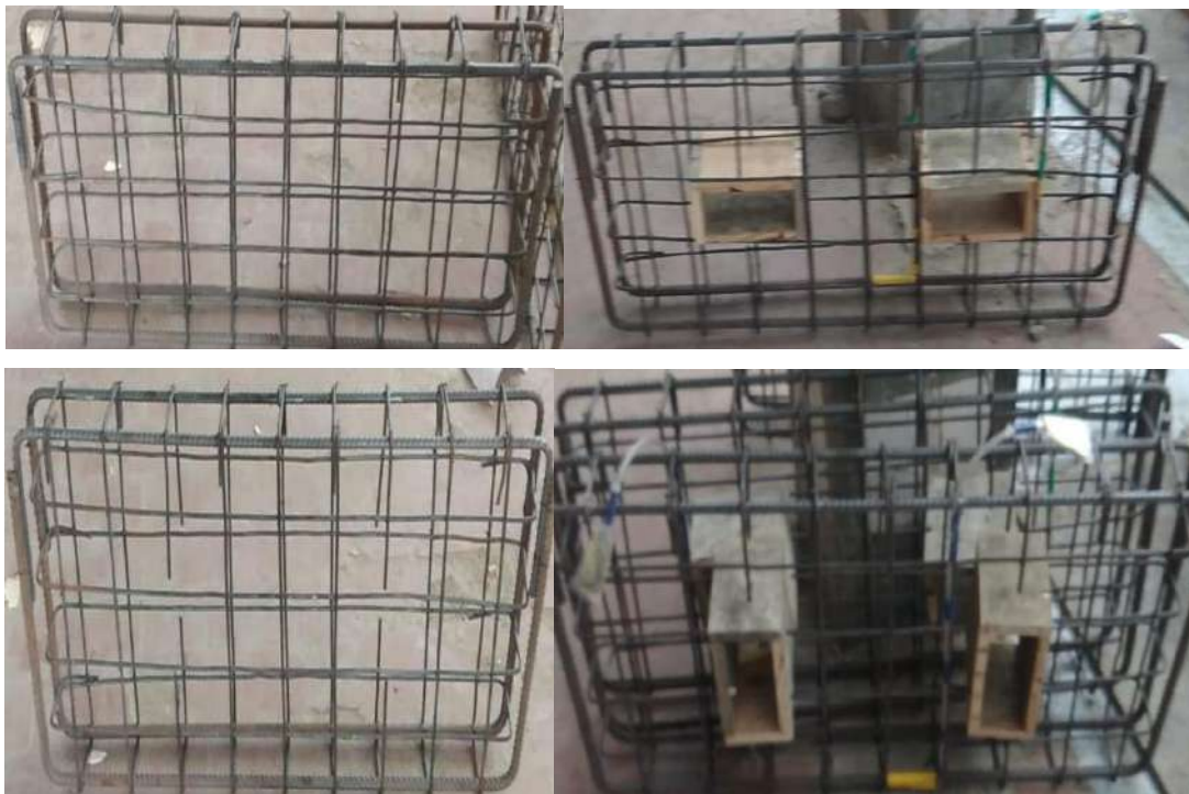
Figure (3- 13): Reinforcement details of deep beams
