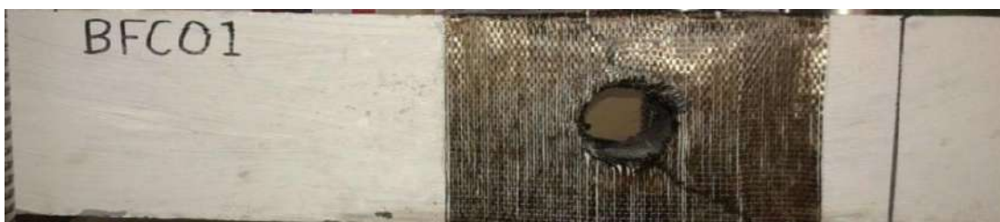
Figure (2-20): Crack pattern of strengthened beam with one circular opening.
