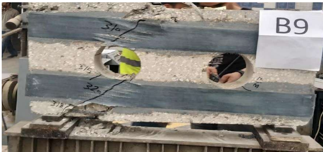
Figure (4-9): Crack pattern of beam B9 at failure
