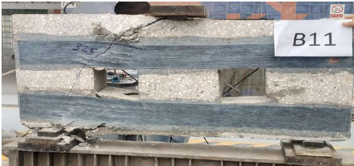
Figure (4-11): Crack pattern of beam B11 at failure
