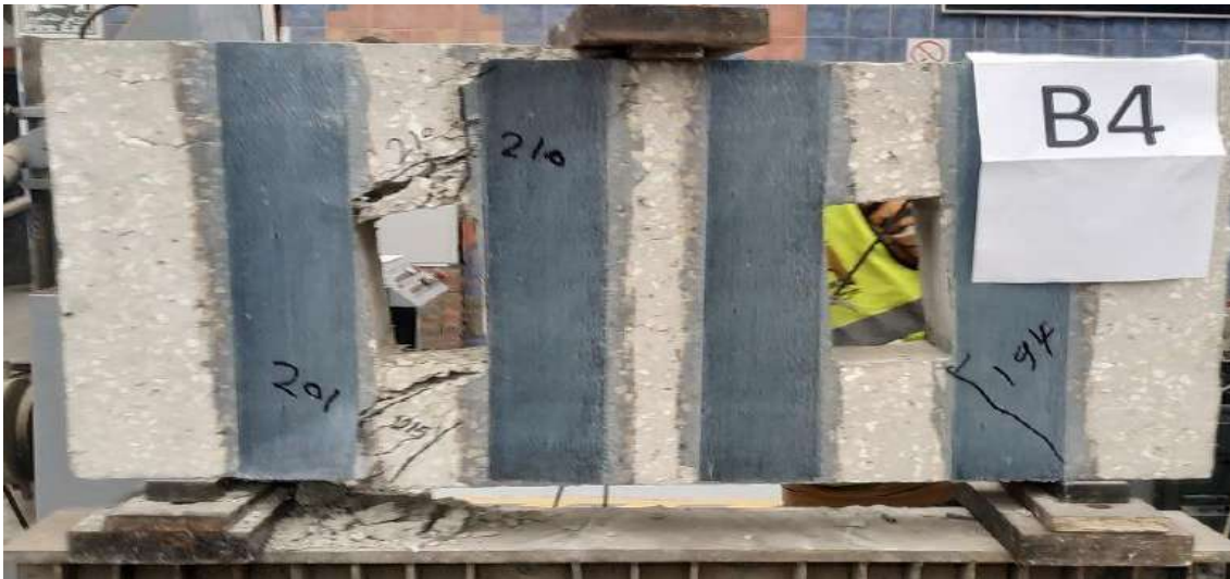
Figure (4-4): Crack pattern at failure (B4)
