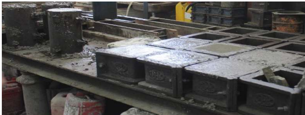
Figure (3-19): The cubes and cylinders after casting and leveling the surface.
