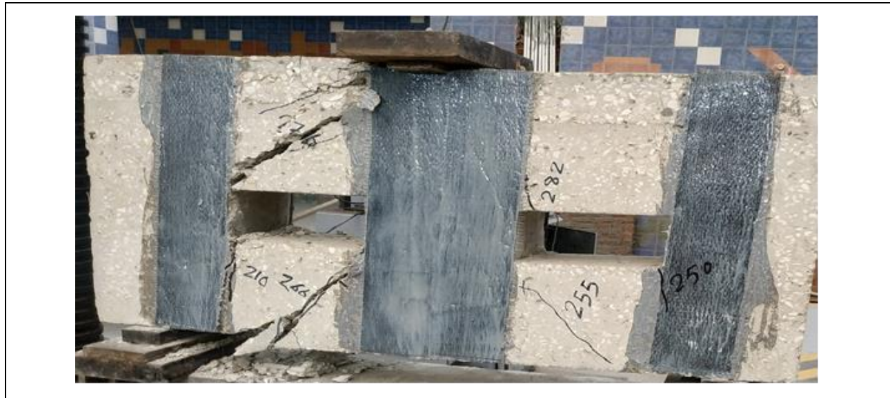
Figure (7): crack patten of deep beam with horizontal openings strengthened with vertical BFRP (VS-HRO)
