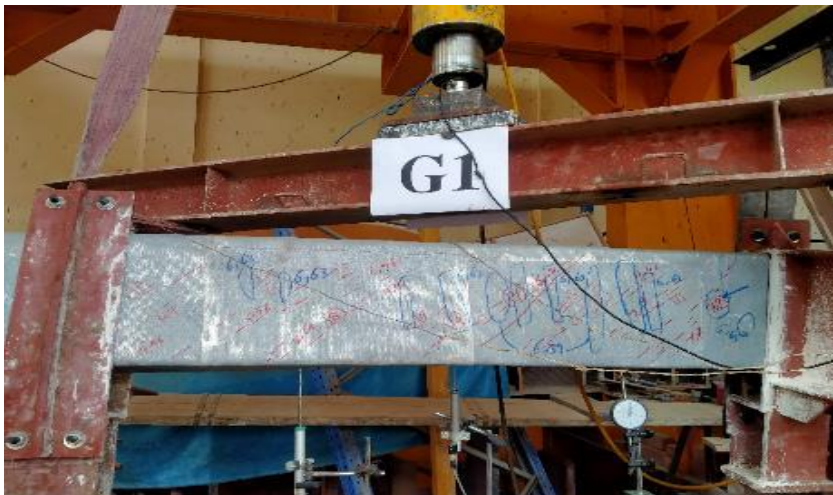
Figure 11 :Fully Wrapped beam after Cracking .
