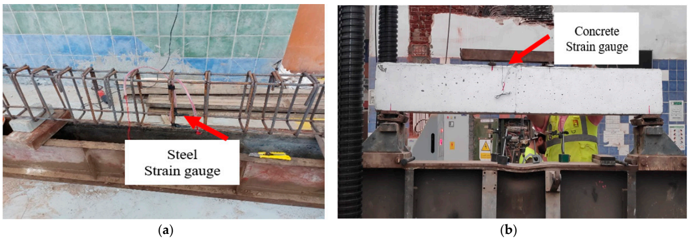
Figure 6. Locations of the strain gauges on (a) steel bars and (b) concrete.
