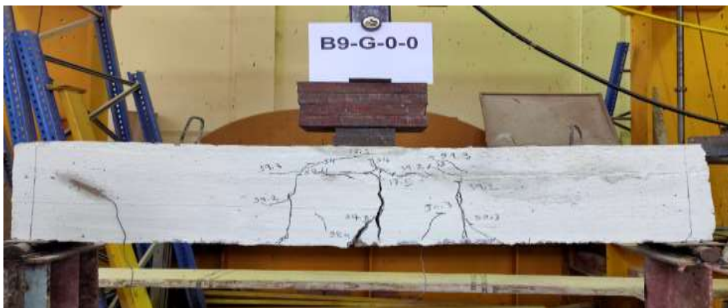
Figure (4): Cracks for Beam (G-0-0) at Failure
