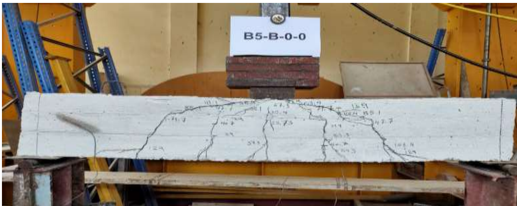
Figure (3): Cracks for Beam (B-0-0) at Failure
