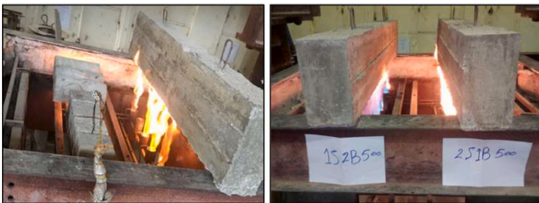
Fig. 5. Beams, Cubes, and Cylinders subjected to Fire.
