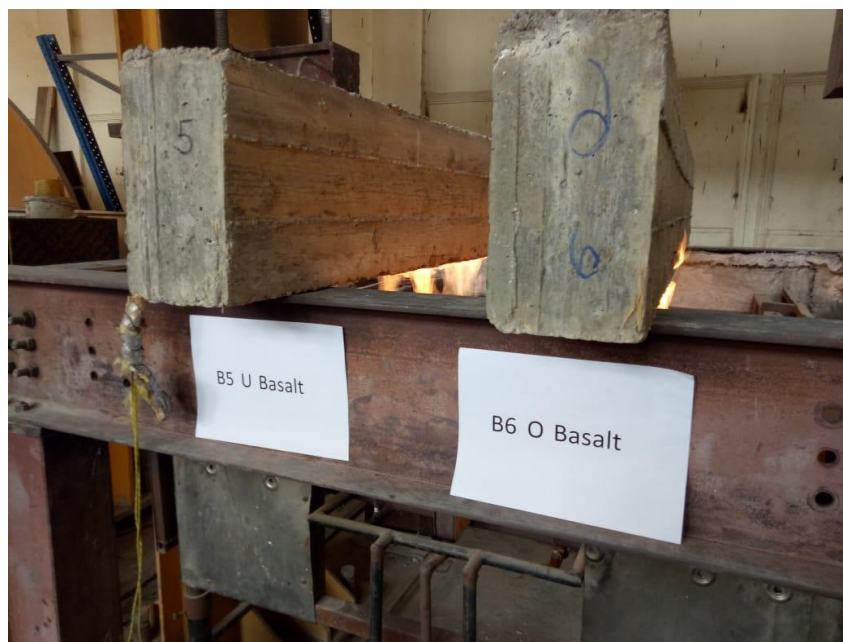
Fig. (3): Burning Beams on 400c.
