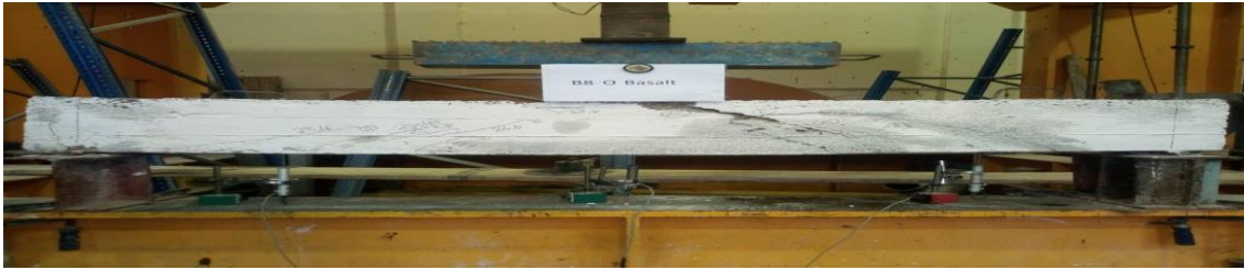
Fig.(17).Cracking Pattern for Beam (B8OB).
