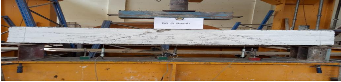
Fig.(16).Cracking Pattern for Beam (B6OB).
