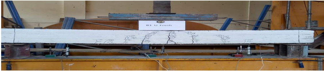
Fig. (6).Cracking Pattern for Beam (B1UF).
