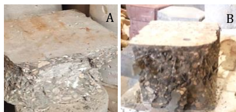
Fig.9 Concrete Cube Compressive Strength Test. (A) without Steel Fiber (B) with Steel Fiber
