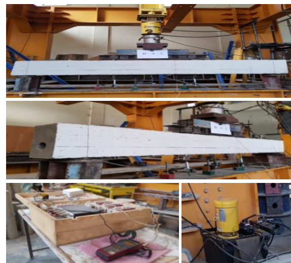
Fig. 16 Beam Test Setup, Dial Gauge and Load Cell
