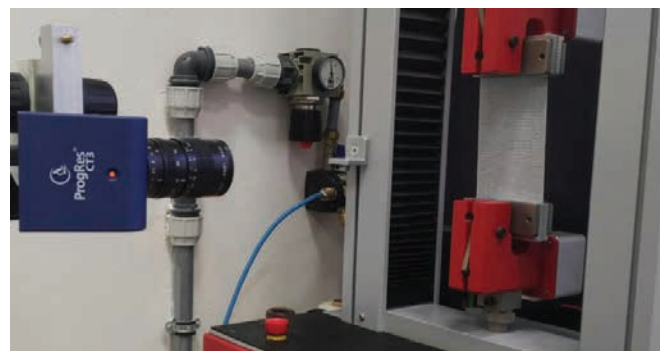
Figure 8. Setup of Testometric M350-5CT instrument and high-speed camera
