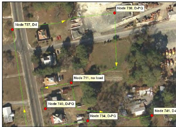
Arrows indicating current flow direction and node/load identification.
