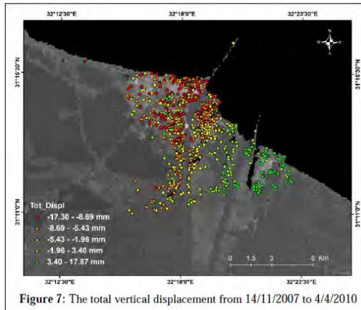
Figure 7: The total vertical displacement from 14/11/2007 to 4/4/2010
