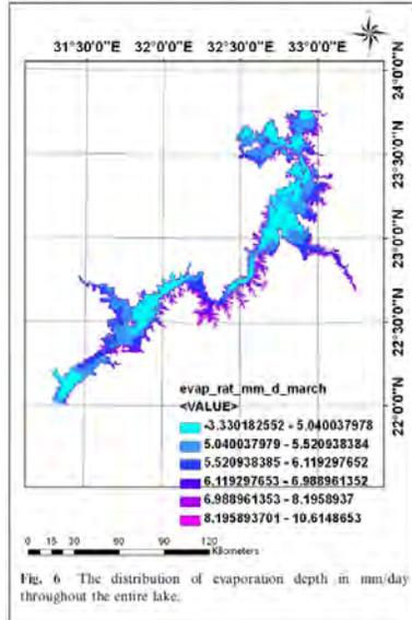
Fig. 6 The distribution of evaporation depth in mm/day throughout the entire lake.
