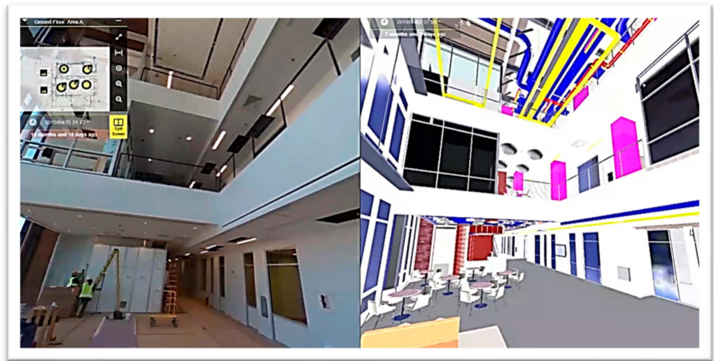
Figure 6. Construction Documentation Using HOLOBUILDER Platform. The left image is captured using 360° cameras. The right side indicates the same scene in the BIM model.
