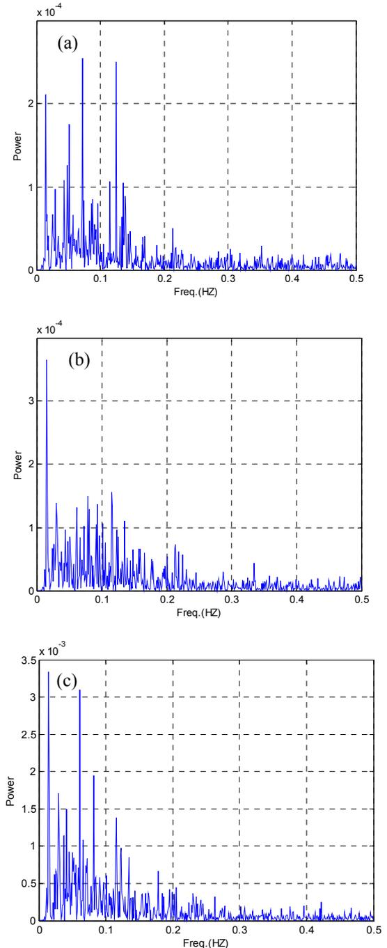
Figure 4. Dynamic frequency displacement modes in directions a) x; b) y and c) z
