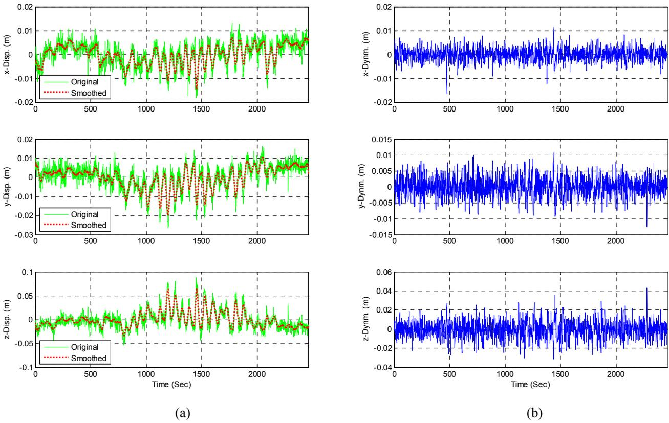
Figure 2. a) Apparent displacement (original) and extracted semi static (smoothed) displacement; b) extracted dynamic displacement from RTK-GPS observations
