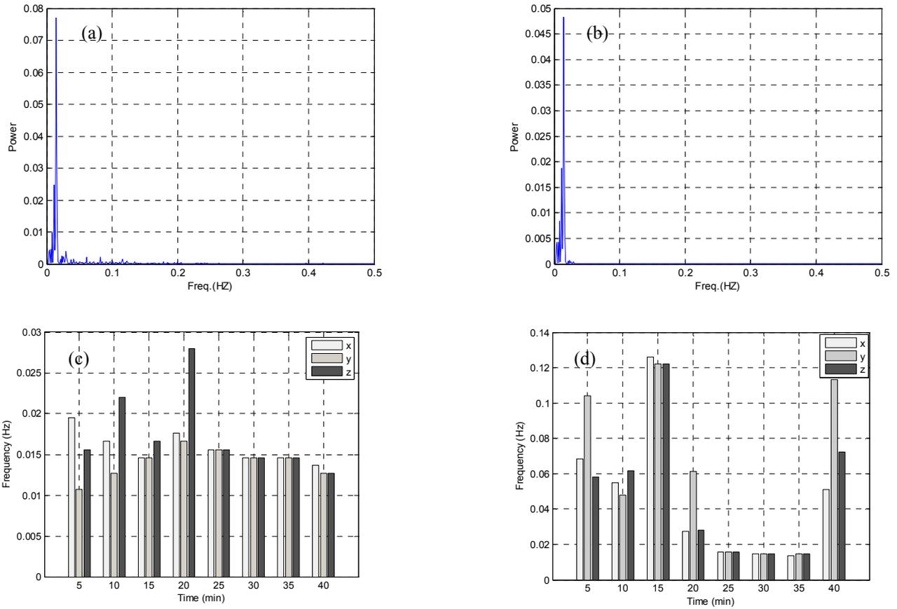
Figure 3. a) z-apparent frequency; b) z-semi static frequency; c) time frequency semi static displacement; d) time frequency dynamic displacement
