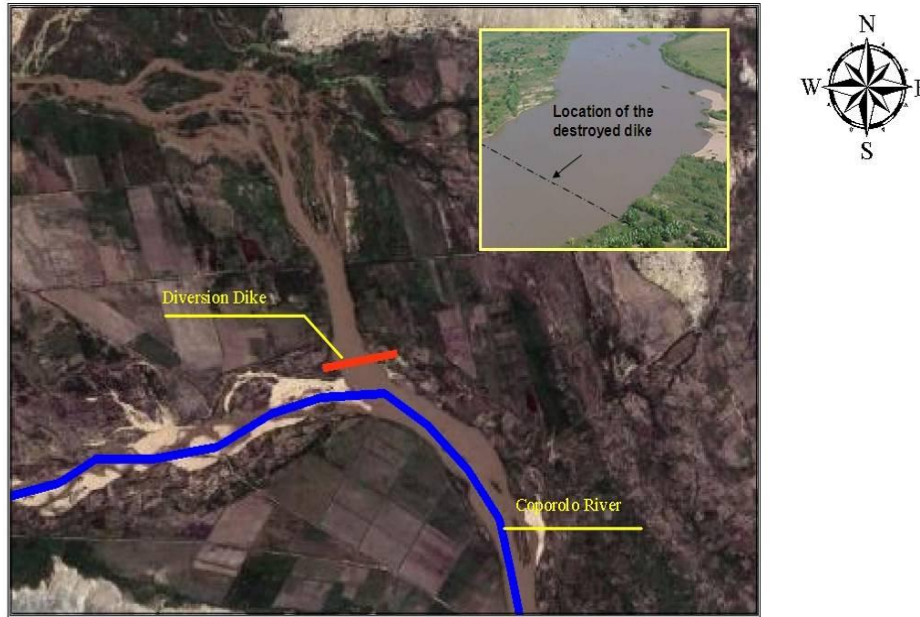
Figure 8: Proposed diversion dike
