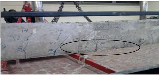
Figure 5 Failure and crack pattern of control specimen B1.
