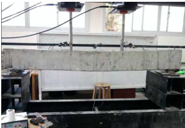
Figure 4 Set-up for four-point bending test in laboratory.
