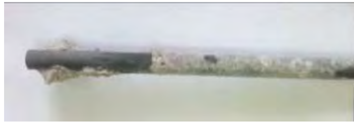
Figure 10 Debonded CFRP bar
