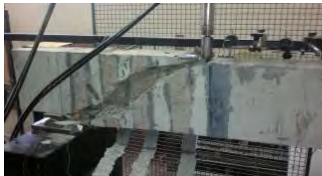
Figure 8 Crack patterns of specimen S-EBR
