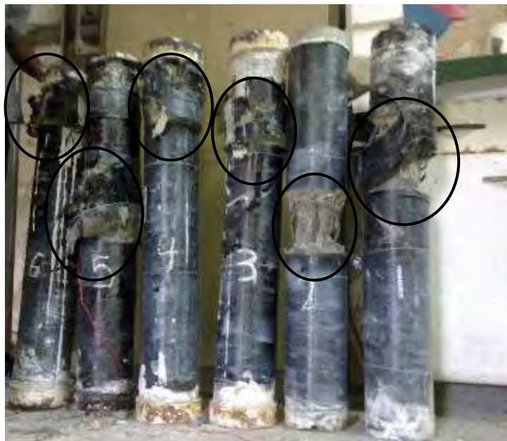
Figure (6) Failure modes for all columns
