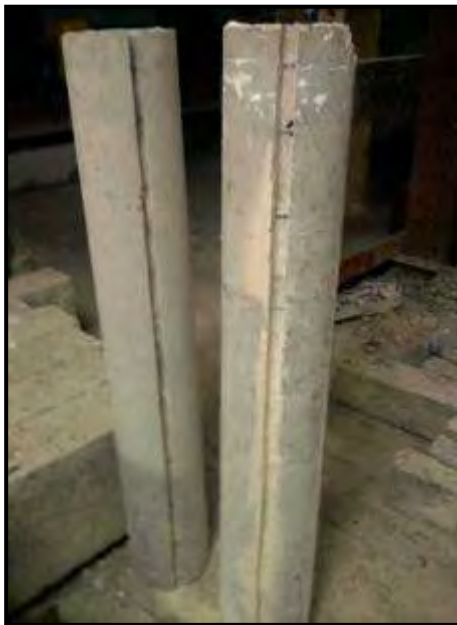
Figure (5) embedding the external reinforcement into the column concrete cover
