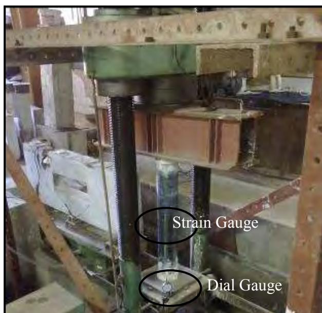
Figure 3. Test Setup and column instrumentation
