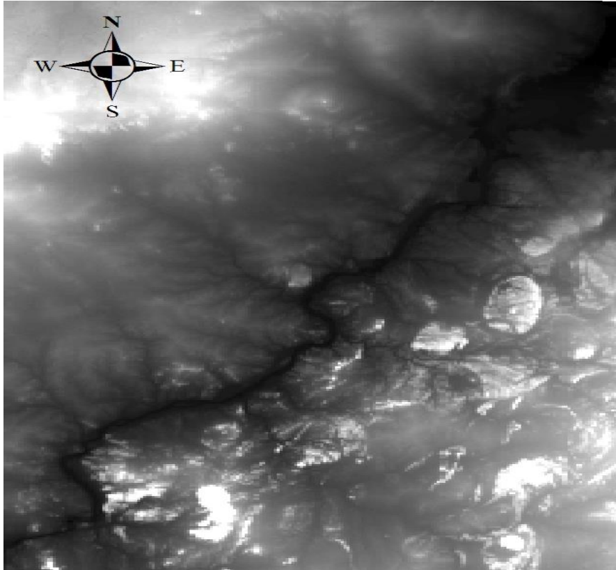
Figure 5: A 90 meters cell size SRTM digital elevation model
