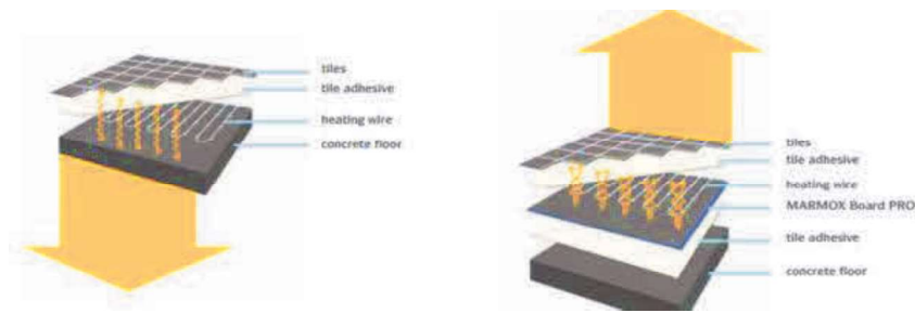
Fig.21. Marmox underfloor heating system. (Marmox Board- http://marmoxboard.com/ZA/marmox_board_pro.html )
