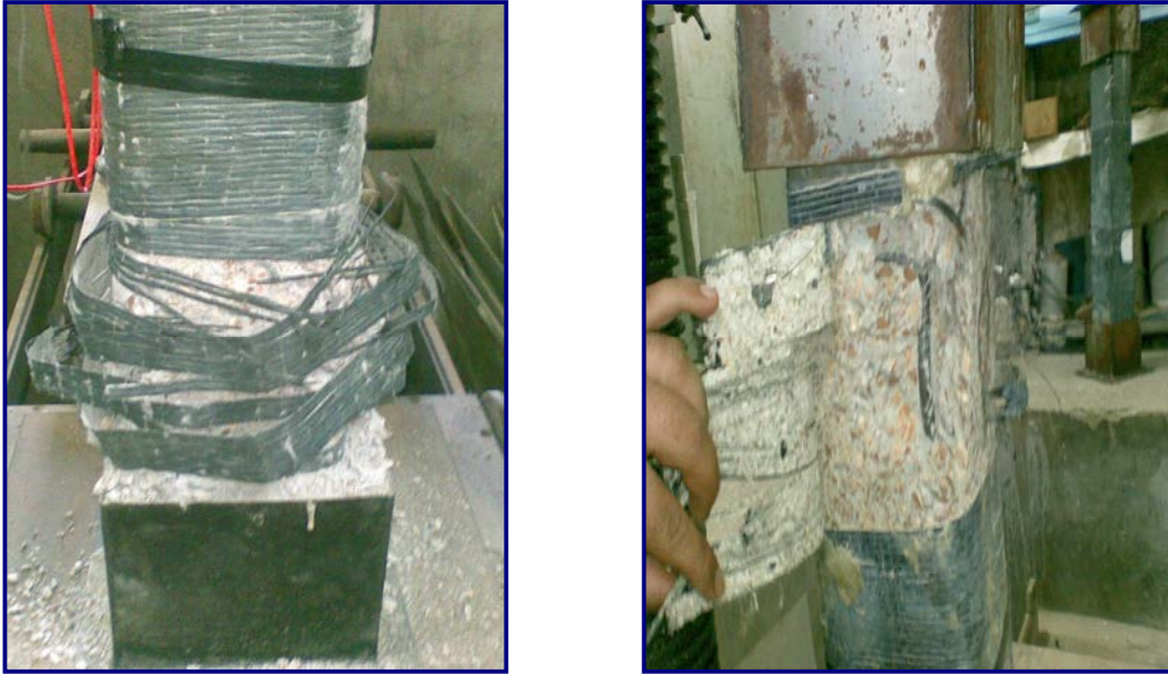
Fig. 4.4 Failure in Columns C.F.-90-24, and R.W.-100-24
