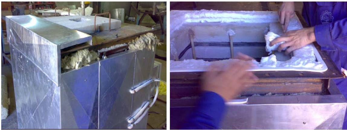
Fig. 3.13 External insulation for walls and roof
