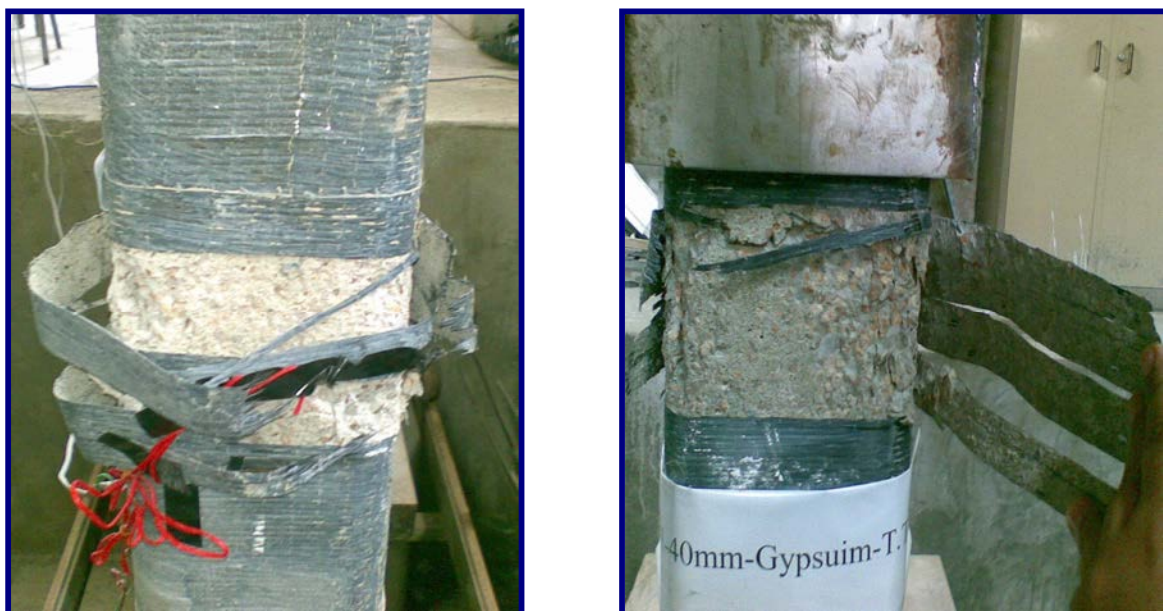
Fig. 4.3 Failure in Columns T.C.-70-24, and G-80-24
