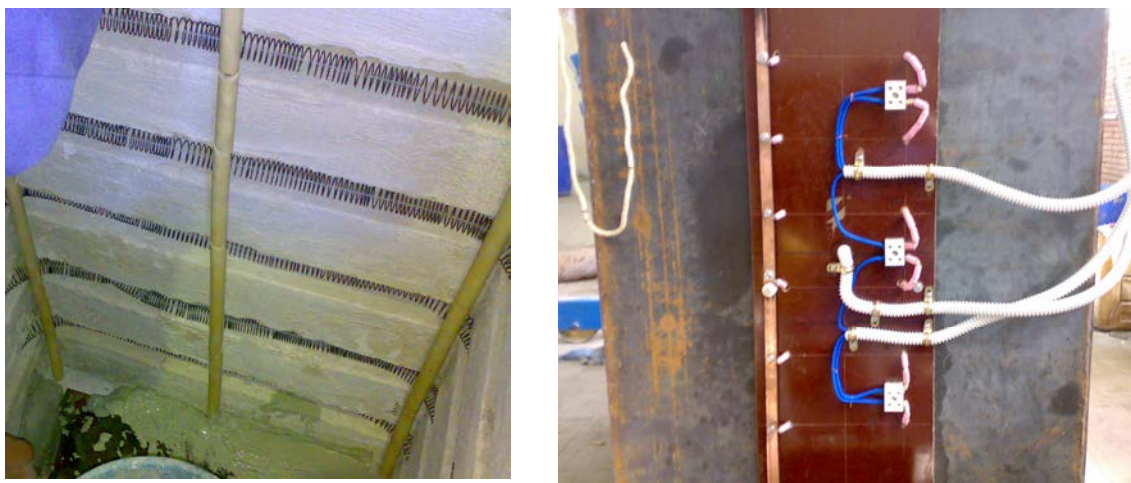
Fig. 3.12 Electric coils insides grooves and electric circuit
