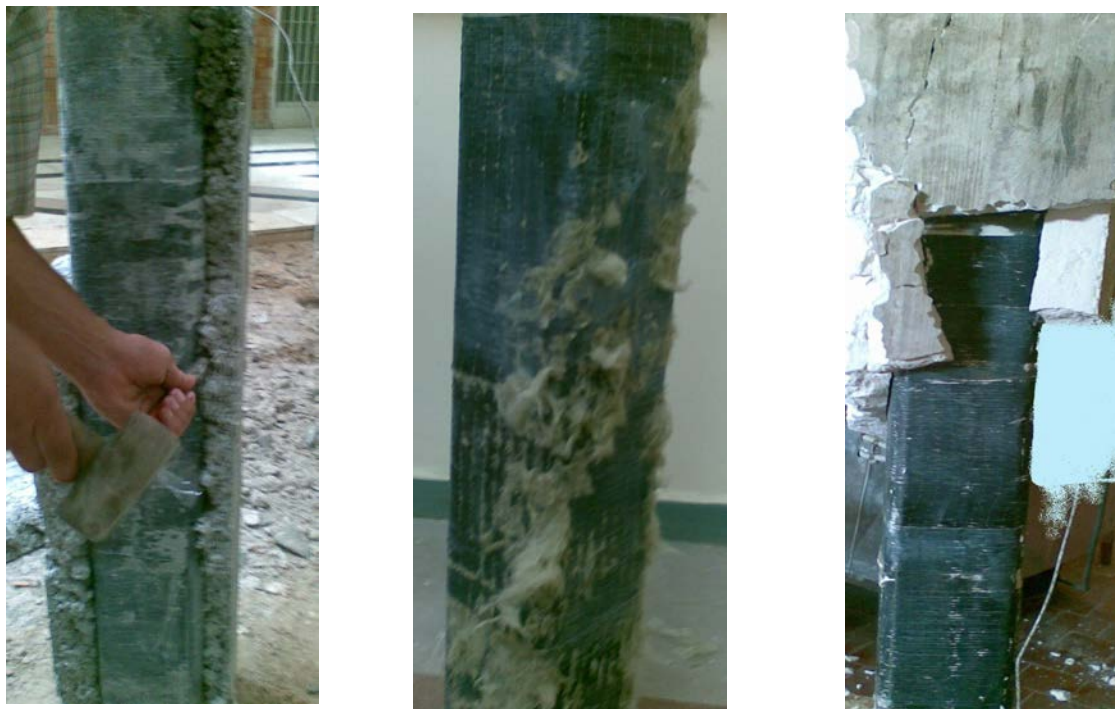
Fig. 4.23 CFRP surface while removing insulating material after subjecting to 100°C
