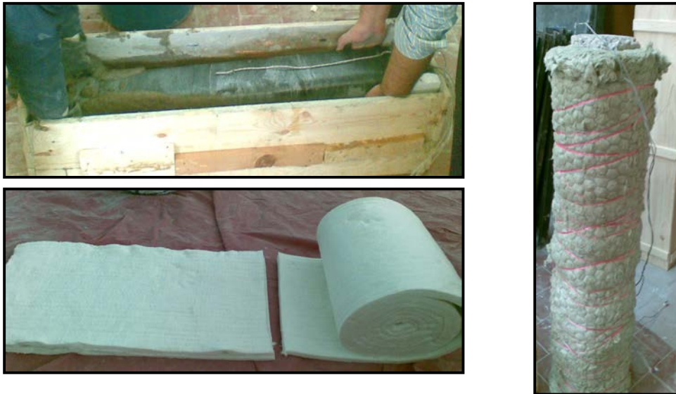
Fig. 3.9 Insulating the tested Columns using different insulating materials.
