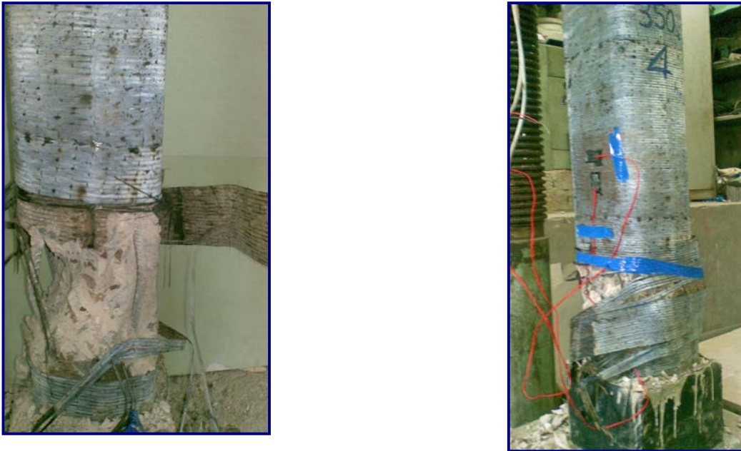
Fig. 4.13 Failure in Column U-350-4
