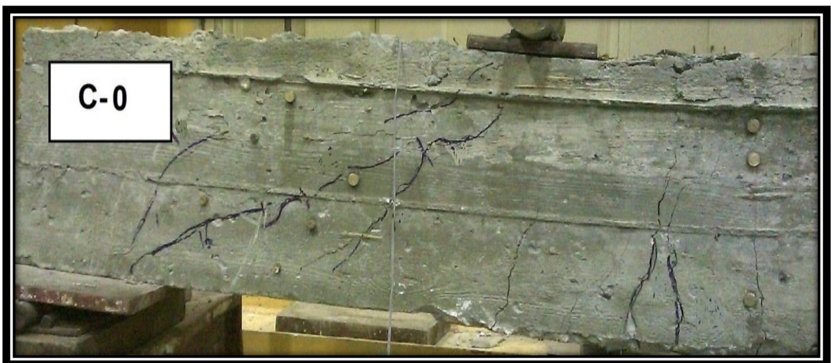
Fig (4.25) Crack Patterns for specimen (C-0).
