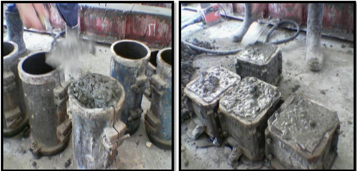
Fig (3.7). Casting the Standard Cubes and Cylinder
