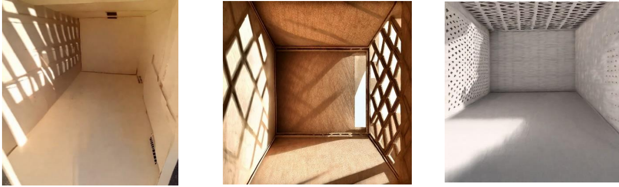
Figure 20: Examples of laser-cut fenestration pattern scale models and their perspective shadow studies in natural light. (Representative sample) [Authors]
