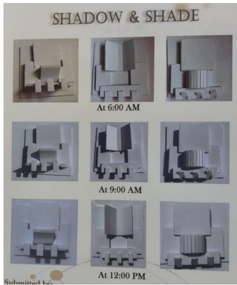
Figure 18: Handmade scale models crafted by the students to study the shadow composition in forms derived from the 3D shadow studies conducted in SketchUp [Authors]
