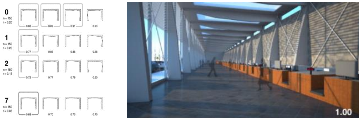
Fig. 13 (Left) Design exploration of structural frames for airport hall design based on performance. (Right) a visual illustration for the structure conceptual design based on algorithmic exploration. [18]
