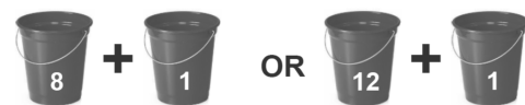
Figure 2. Cement soil ratio according to the Brazilian Standards. Source: ABNT (2012) NBR 10833 & ABCP (1986).
