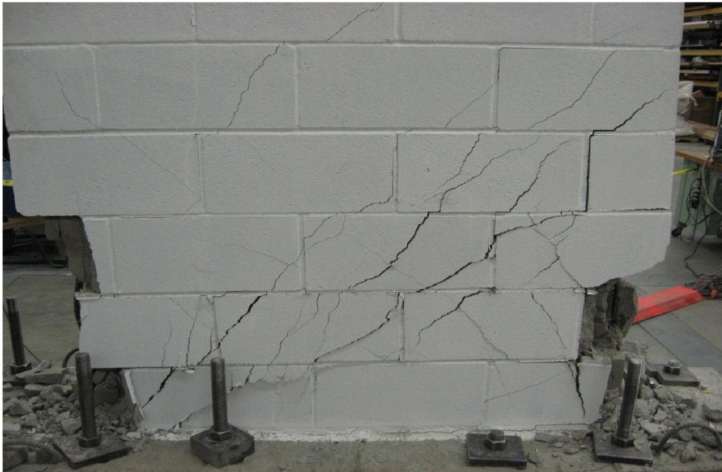
Figure 1.22- Further Development of flexure cracks, (Dg2). (Wall 2, C-Kapoi, 2012)
