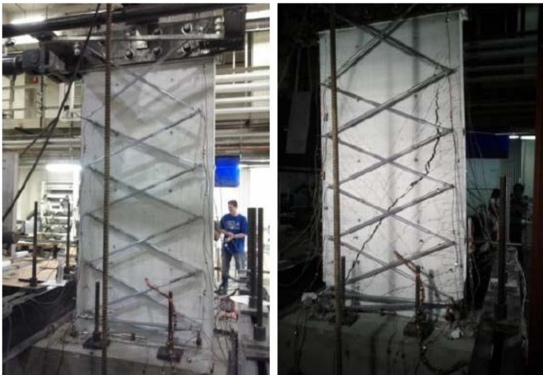
Figure 1.26- Shear Failure, Specimen (1) (Felipe Cifelli, 2011)
