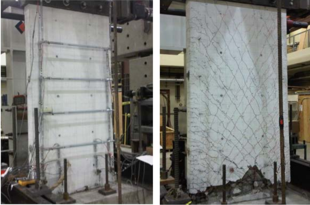
Figure 1.20- Typical flexural failure for reinforced concrete shear wall. Specimen (2) (Felipe Cifelli, 2011) before testing began (Face A). Right: Specimen after loss of lateral load capacity.
