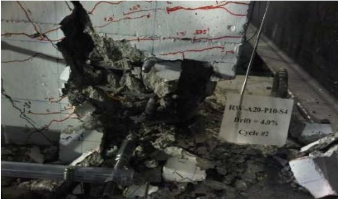
Figure 1.27- Lower right side of specimen after failure, Specimen (1) (Felipe Cifelli, 2011).
