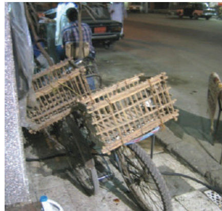
Fig.121. Carrying crates made with date palm midribs. (Photo by Murphy and Richmond 2003)
