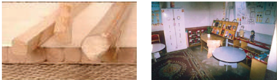
Fig.124. Blockboard made with date palm leaves' midribs (DPLM). Left, the midribs are used as a core while surface veneers are glued on both sides. The total thickness is one cm. Right, Furniture made with DPLM blockboard in a community school established by the UNICEF. (From EGYCOM homepage: www.egy-com.org )
