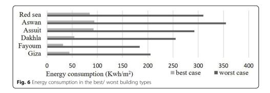
under investigation reduced the thermal discomfort hours, raising the efficiency of the built environment and the Energy consumption decreased from 35 to 50%. Therefore, building with compressed stabilized earth block is an environmentally sustainable solution applied in residential areas in the villages of Upper Egypt to reduce deficiencies in environmental adaptation. Therefore, the research hypothesis is right.
