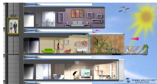
Fig. 4-11 Using photovoltaic panels between the tower's floors
