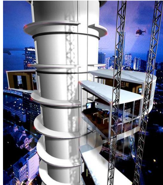
Fig. 4-10 An illustration of how the single modules are assembled around the core of the tower.
