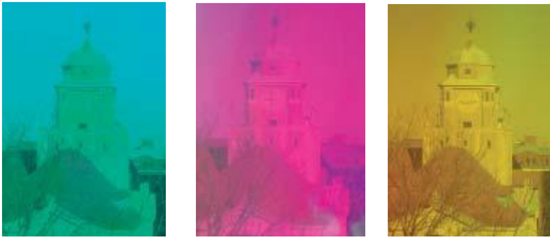
Fig. 3-7 Radiant mirror film. The color of the transparent film depends on the angle of the viewer with respect to the film.
