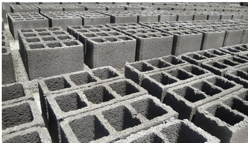
Figure 3.4: Hollow concrete blocks with which local work crews in the Gaza Strip are well versed.
