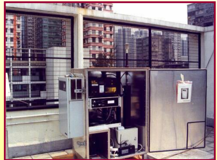
tapered element oscillating microbalance - continuous RSP
